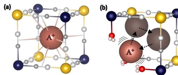
Fig. 3 Scheme of (a) the closed and (b) the open  $\text{Co}(\text{Co}(\text{OH}_2)_3\text{Fe}_3$  Cavities and the proposed positioning for the bigger alkali cations ( $\text{Rb}^+$ ,  $\text{Cs}^+$ ) in each of them.
