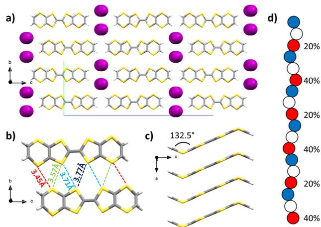
Fig. 2 X-ray crystal structure of  $(\text{BVDT-TTF})_{2.5}(\text{I}_3)$  (a) viewed along the  $a$  axis. Details showing (b) the intermolecular S–S distances between two molecules from adjacent stacks viewed along the  $a$  axis, (c) a side-view along the  $b$  axis of a single stack of **BVDT-TTF** and (d) a schematized view of the disorder of the triiodide counter-anions along the  $b$  axis (carbon: grey; sulphur: yellow; iodine: purple; hydrogen: white).
