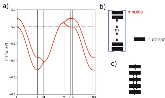
**Fig. 7** (a) Band structure for the hypothetical metallic state of  $(\text{BVD-TTF})_{2.5}(\text{I}_3)$  where  $\Gamma = (0, 0, 0)$ ,  $X = (a^*/2, 0, 0)$ ,  $Y = (0, b^*/2, 0)$ ,  $Z = (0, 0, c^*/2)$ ,  $M = (a^*/2, b^*/2, 0)$  and  $N = (a^*/2, 0, c^*/2)$ . Discrete (donor<sub>m</sub>)<sup>n+</sup> (b) and (donor<sub>s</sub>)<sup>2+</sup> (c) units discussed in the text.
