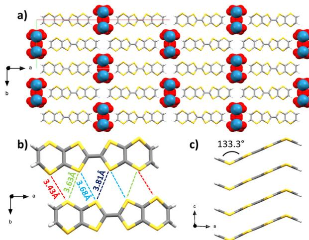
Fig. 3 X-ray crystal structure of  $(\text{BVDT-TTF})_2(\text{ReO}_4)$  (a) viewed along the  $c$  axis. Details showing (b) the intermolecular S–S distances between two molecules from adjacent stacks viewed along the  $c$  axis, and (c) a side-view along the  $b$  axis of one stack of **BVDT-TTF** (carbon: grey; sulphur: yellow; rhenium: blue; oxygen: red; hydrogen: white).
