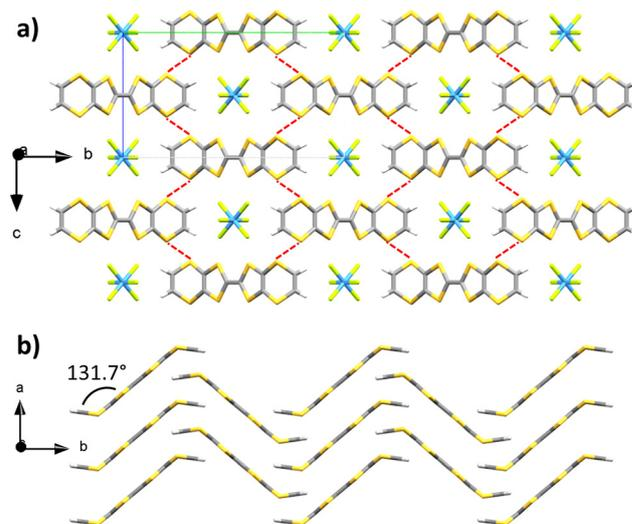
Fig. 1 X-ray crystal structure of **BVD-TTF**( $\text{TaF}_6$ ) viewed along (a) the *a* axis and (b) the *c* axis (carbon: grey; sulphur: yellow; tantalum: blue; fluorine: green; hydrogen: white). For the sake of clarity the  $\text{TaF}_6^-$  anions have been removed on (b).
