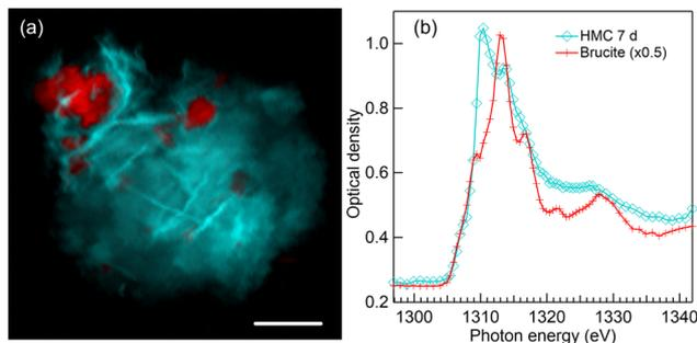
**Fig. 6** (a) Color composite map of STXM recording at Mg K-edge of precipitates formed after 7-day reaction time in water. HMC crystals are shown in light blue and residual brucite in red. (b) Extracted XANES spectra used to fit the color composite map shown in (a): unreacted brucite (red line with crosses) and HMC (light blue line with diamonds). Scale bar is 2  $\mu\text{m}$ .
