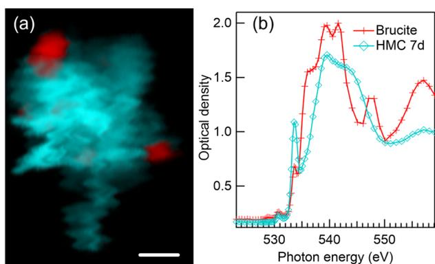
**Fig. 7** (a) Color composite map of STXM recording at O K-edge of precipitates formed after 7-day reaction time in water. HMC crystals are shown in light blue and residual brucite in red. (b) Extracted XANES spectra used to fit the color composite map shown in (a): unreacted brucite (red line with crosses) and HMC (light blue line with diamonds). Scale bar is 1  $\mu\text{m}$ .
