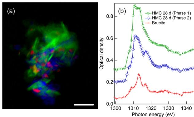
**Fig. 9** (a) Color composite map of precipitates formed after 28-day of reaction in water. Brucite areas are depicted in red, and two HMC phases in green and blue. (b) Corresponding Mg K-edge XANES spectra extracted from the measured precipitate agglomerate showing brucite with a red line with crosses, a dypingite-like HMC phase with a green line with spheres and an undefined HMC phase with a blue line with diamonds. Scale bar 2  $\mu\text{m}$ .
