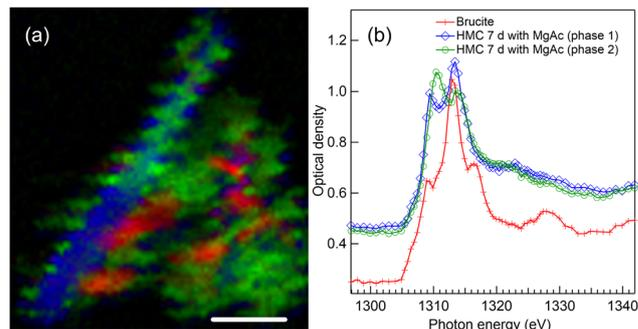
**Fig. 8** Color composite map of STXM recording at Mg K-edge of precipitates formed after 7-day reaction time with Mg-acetate. Brucite is shown in red and two HMC phases with blue and green. (b) Extracted XANES spectra used to fit the color composite map shown in (a): unreacted brucite (red line with crosses) and HMC phases 1 and 2 (blue line with diamonds and green line with spheres). Scale bar is 1  $\mu\text{m}$ .
