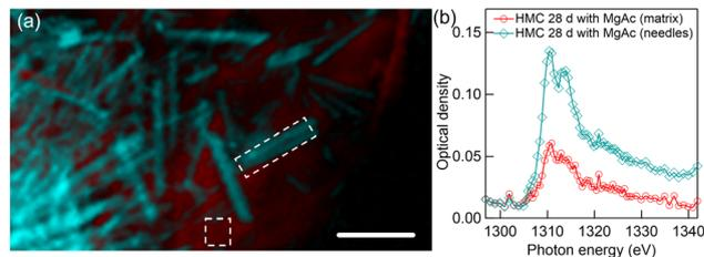
**Fig. 10** (a) Color composite map of STXM recording at Mg K-edge of precipitates formed after 28-day reaction time with Mg-acetate. Slightly absorbing matrix is shown in red and HMC needles with light blue. (b) XANES spectra used to fit the color composite map extracted from regions shown with dashed rectangles in (a): matrix (red line with spheres) and HMC (light blue line with diamonds). Scale bar 2  $\mu\text{m}$ .
