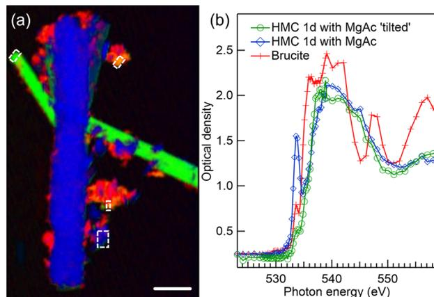
**Fig. 5** (a) Color composite map of STXM recording at O K-edge of precipitates formed after 1 day reaction time in presence of Mg-acetate. HMC crystals are shown in blue and green and residual brucite in red. (b) XANES spectra of unreacted brucite (red line with crosses) and thin HMC agglomerate (blue line with diamonds). Regions from which spectra were extracted are shown with dashed rectangles in (a) (average of two locations for brucite). Scale bar is 3  $\mu\text{m}$ .
