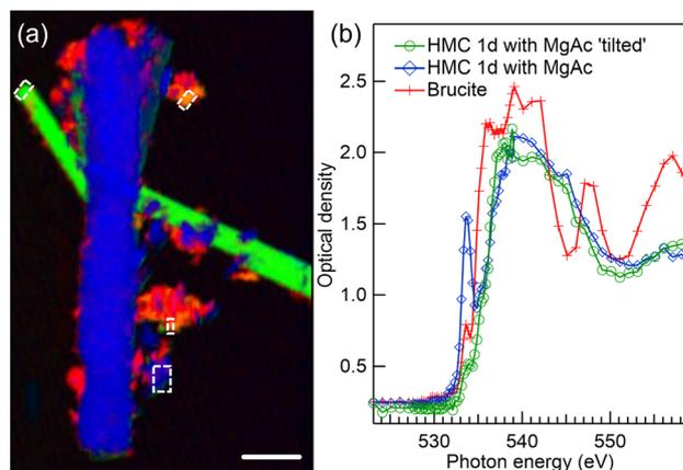
**Fig. 5** (a) Color composite map of STXM recording at O K-edge of precipitates formed after 1 day reaction time in presence of Mg-acetate. HMC crystals are shown in blue and green and residual brucite in red. (b) XANES spectra of unreacted brucite (red line with crosses) and thin HMC agglomerate (blue line with diamonds). Regions from which spectra were extracted are shown with dashed rectangles in (a) (average of two locations for brucite). Scale bar is 3  $\mu\text{m}$ .
