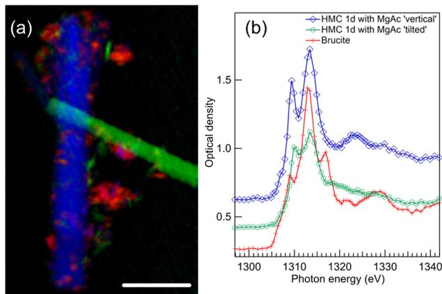
**Fig. 4** (a) Color composite map of STXM recording at Mg K-edge of precipitates formed after 1 day reaction time in presence of Mg-acetate. HMC crystals are shown in blue and green and residual brucite in red. (b) Corresponding XANES spectra of selected regions of unreacted brucite (red line with crosses), vertical crystal (blue line with diamonds), and 25° tilted crystal (green line with spheres). Scale bar 5  $\mu\text{m}$ .
