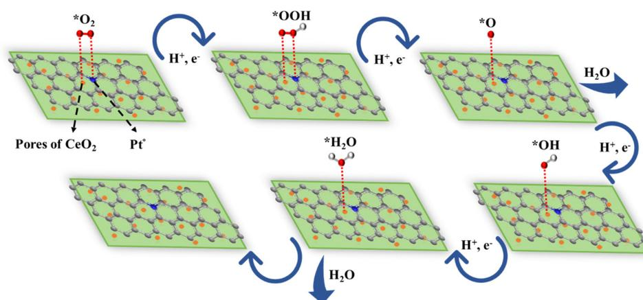
Fig. 7 Mechanism of ORR on the surface of Pt@CoO<sub>x</sub>/NC@CeO<sub>2</sub>1.
