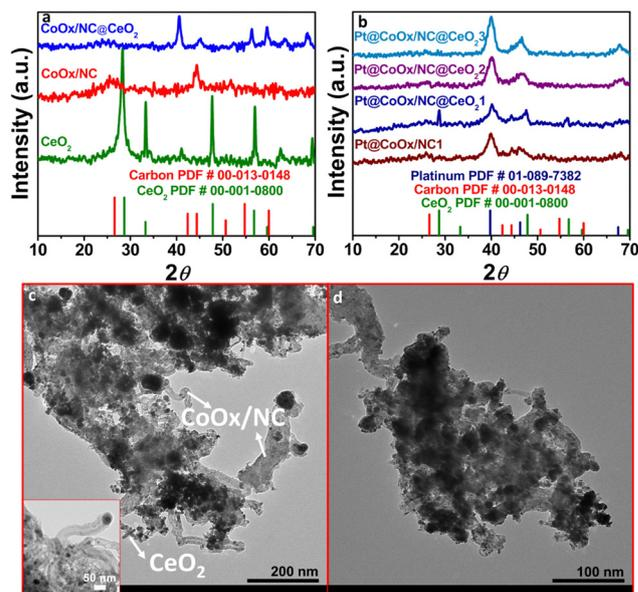
Fig. 1 (a) X-ray diffraction pattern of CeO<sub>2</sub>, CoO<sub>x</sub>/NC and CoO<sub>x</sub>/NC@CeO<sub>2</sub>. (b) X-ray diffraction pattern of Pt@CoO<sub>x</sub>/NC1 and Pt@CoO<sub>x</sub>/NC@CeO<sub>2</sub>s. (c) TEM analysis of Pt@CoO<sub>x</sub>/NC@CeO<sub>2</sub>1 at 200 nm. (d) TEM analysis of Pt@CoO<sub>x</sub>/NC@CeO<sub>2</sub>1 at 100 nm.
