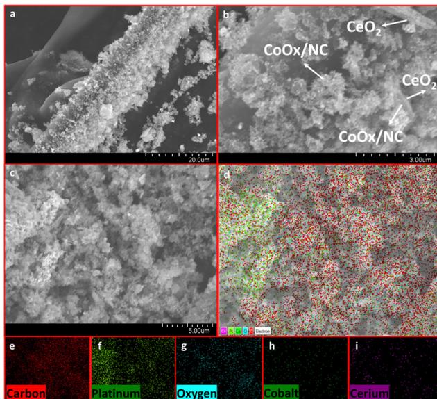
Fig. 2 SEM analysis of Pt@CoO<sub>x</sub>/NC@CeO<sub>2</sub>1: (a) 20 μm, (b) 3 μm and (c) 5 μm; (d) elemental mapping of Pt@CoO<sub>x</sub>/NC@CeO<sub>2</sub>1; (e) carbon, (f) platinum, (g) oxygen, (h) cobalt and (i) cerium.
