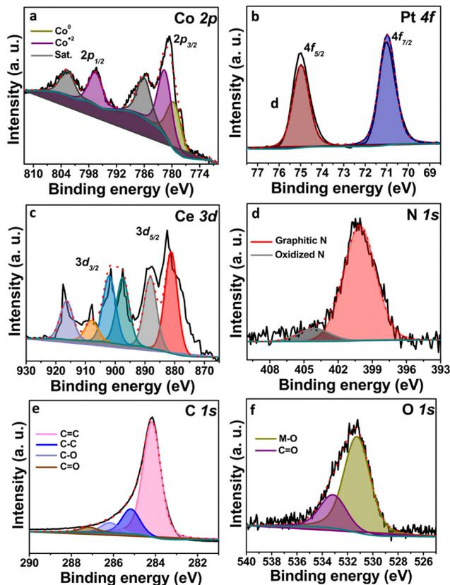
Fig. 3 XPS of Pt@CoO<sub>x</sub>/NC@CeO<sub>2</sub>1: (a) Co 2p, (b) Pt 4f, (c) Ce 3d, (d) N 1s, (e) C 1s and (f) O 1s.
