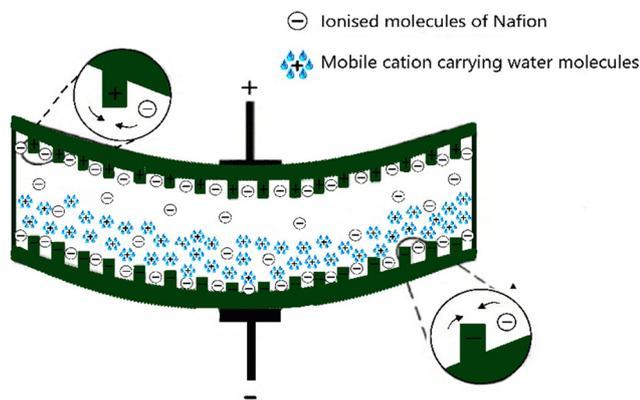
Fig. 4 Schematic diagram of the coulombic force interaction of an IPMC.<sup>17</sup>
