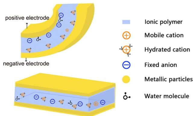
Fig. 2 Schematic diagrams of the hydration cation migration effect of an IPMC.<sup>15</sup>
