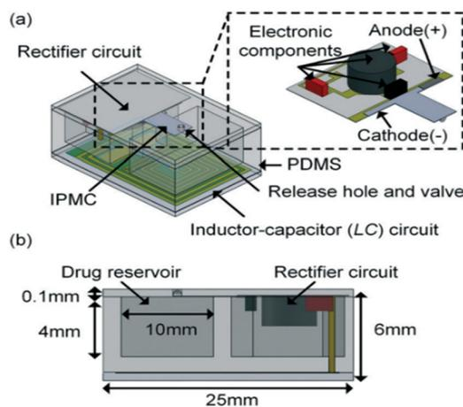
Fig. 9 IPMC-based cantilever valve for drug delivery. The body of the device is made of biocompatible polydimethylsiloxane (PDMS) and has external dimensions of 15 mm  $\times$  25 mm  $\times$  6 mm, including drug storage with a maximum loading capacity of 520  $\mu\text{L}$ . (a) Schematic illustration of the drug delivery device; (b) side view of the drug delivery device. Reproduced with permission.<sup>95</sup> Copyright 2018 Royal Society of Chemistry.
