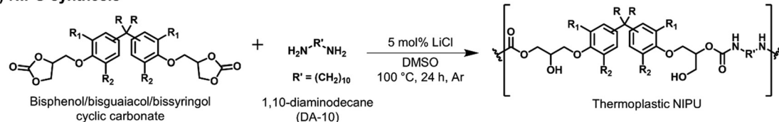
Scheme 1 Synthesis of (a) BGF/BSF using guaiacol/syringol and vanillyl/syringyl alcohol, (b) BGA/BSA using guaiacol/syringol and acetone, (c) diglycidyl ether of bisguaiacol/bisysyringol from respective bisguaiacol/bisysyringol and epichlorohydrin, (d) bisguaiacol/bisysyringol cyclic carbonate from respective diglycidyl ether and CO 2 , and (e) NIPU using respective bisguaiacol/bisysyringol cyclic carbonate and 1,10-diaminodecane (DA-10).
