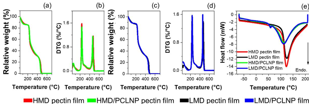
Fig. 4 Thermogravimetric (a)–(d) and differential scanning calorimetric (e) curves of high (HMD – red line) and low (LMD – black line) pectin films and incorporated with poly ( $\epsilon$ -caprolactone) (green and blue line, respectively).
