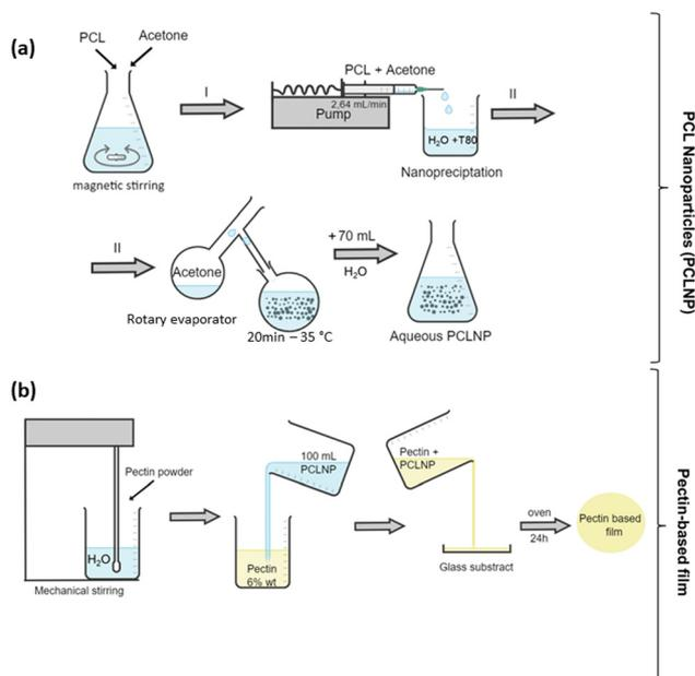
Fig. 1 Illustration of the experimental procedure of the PCL NPs' synthesis (a) by nanoprecipitation and Pectin-based film production (b).
