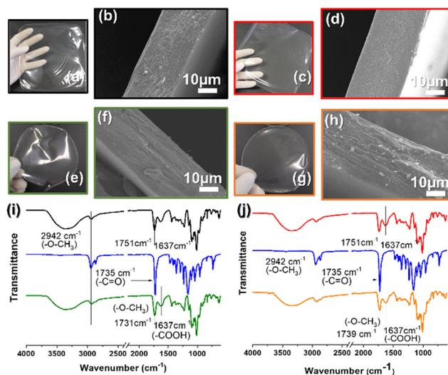
Fig. 3 Digital photographs of control HMD (a) and LMD (c) pectin films and HMD/PCLNP (e), and LMD/PCLNP (g) nanocomposite films. SEM images of the cryo-fractured cross-sections of HMD (b), LMD (d), HMD/PCLNP (f), and LMD/PCLNP (h) films. FT-IR spectra of PCLNP ((i) and (j); blue line), HMD ((i); black line), LMD ((j); red line), HMD/PCLNP ((i); green), and LMD/PCLNP ((j); orange line) films.
