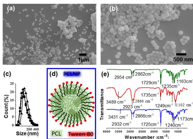
Fig. 2 (a and b) Scanning electron microscopy images of poly( $\epsilon$ -caprolactone) nanoparticles (PCLNPs) at different magnifications. (c) Representation of the size distribution of three different syntheses of poly( $\epsilon$ -caprolactone) (PCL) nanoparticles obtained by dynamic light scattering (DLS). (d) Schematic structure of PCLNPs. (e) FT-IR spectra of PCL (green), Tween 80 (red), and PCLNPs (blue).
