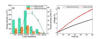
Fig. 8 (a) Energy (bars) and power (line) densities of TENG devices at various load resistances; (b) voltages across the capacitor generated by TENG devices based on PEBA/UiO-66 or PEBA/UiO-66-NH<sub>2</sub> composites in contact with ITO
