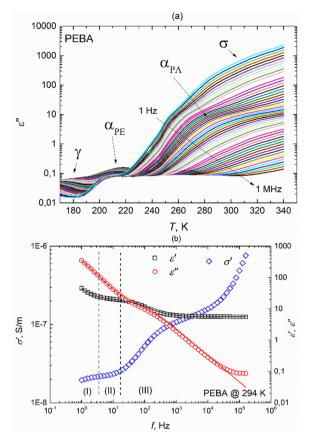
Fig. 3 (a) Temperature dependencies of the imaginary part of the complex dielectric permittivity of the PEBA polymer during heating at different frequencies, (b) frequency dependencies of  $\epsilon'$ ,  $\epsilon''$  and  $\sigma'$  at a temperature of 294 K. Solid lines represent fits according to eqn (2) with an additional term accounting for M-W-S interfacial polarization in the (I) region.
