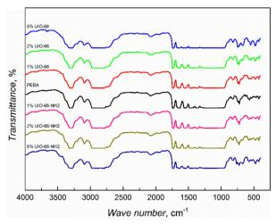
PEBA/UIO-66 PEBA/UIO-66-NH<sub>2</sub> Fig. 1 Infrared spectra composites
