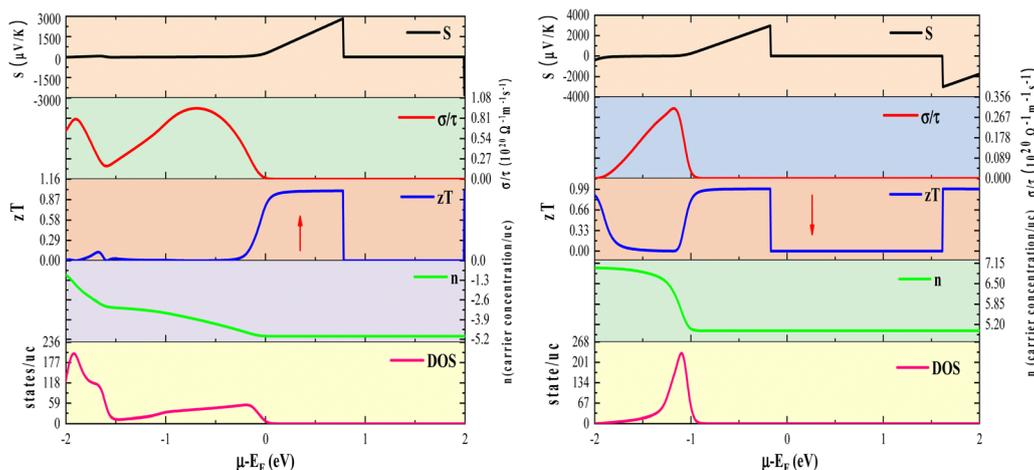
Fig. 13 Comparative variation in Seebeck coefficient ( $S$ ), electrical conductivity ( $\sigma/\tau$ ), figure of merit ( $zT$ ), carrier concentration ( $n$ ) and volumetric density of states (DOS) against chemical potential at 300 K, for the  $\text{K}_2\text{GeMnCl}_6$  halide perovskite (the upward and downward arrows indicate spin-up and spin-down directions, respectively).
