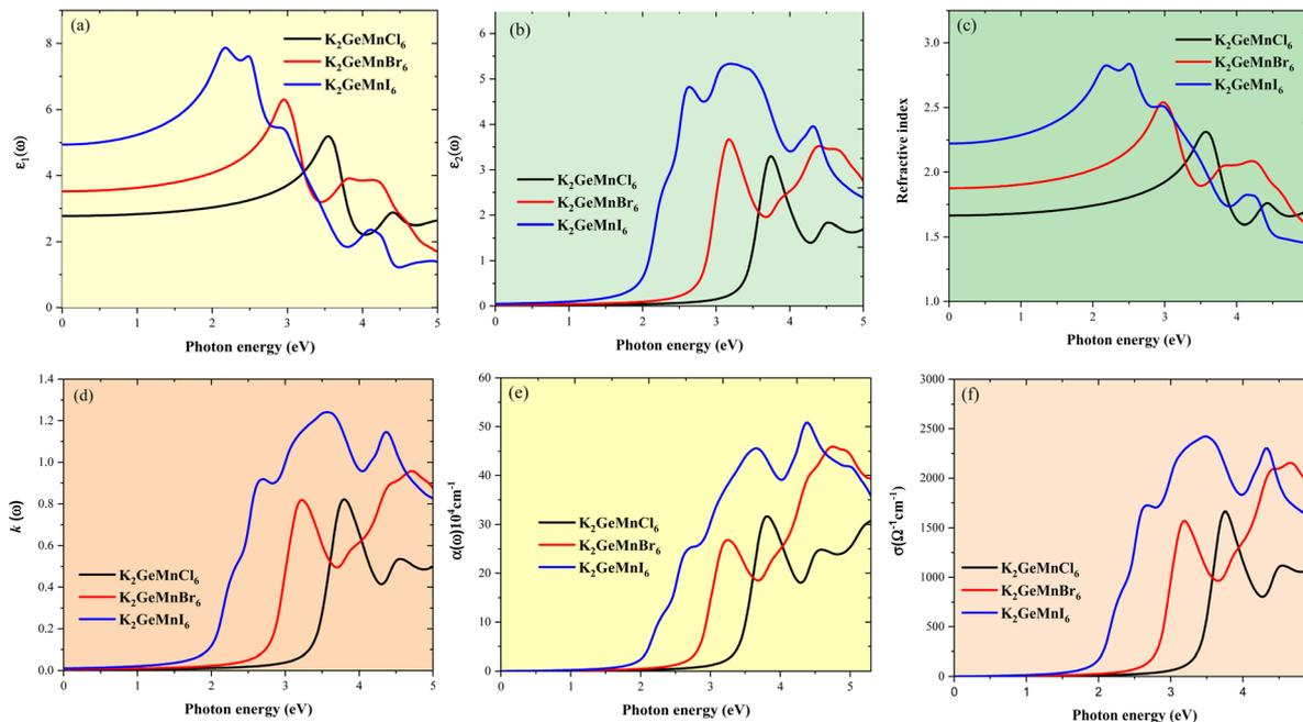
Fig. 10 The computed (a) real part of dielectric ( $\epsilon_1(\omega)$ ), (b) imaginary part of dielectric ( $\epsilon_2(\omega)$ ), (c) refractive index ( $n(\omega)$ ), (d) extinction coefficient ( $k(\omega)$ ), (e) absorption coefficient ( $\alpha(\omega)$ ) and (f) photoconductivity ( $\sigma$ ) for K<sub>2</sub>GeMnX<sub>6</sub> (X = Cl, Br, I) halide perovskites.
