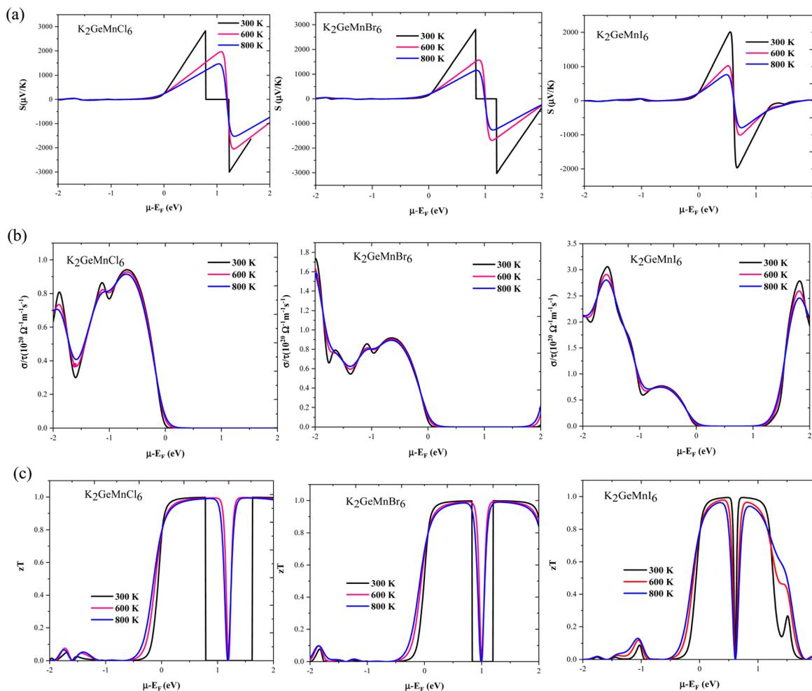
Fig. 12 Thermoelectric plots of (a) Seebeck coefficient ( $S$ ), (b) electrical conductivity ( $\sigma/t$ ), and (c) figure of merit ( $zT$ ) against chemical potential at different temperatures (300 K, 600 K, 800 K) for  $K_2GeMnX_6$  ( $X = Cl, Br, I$ ) halide perovskites.
