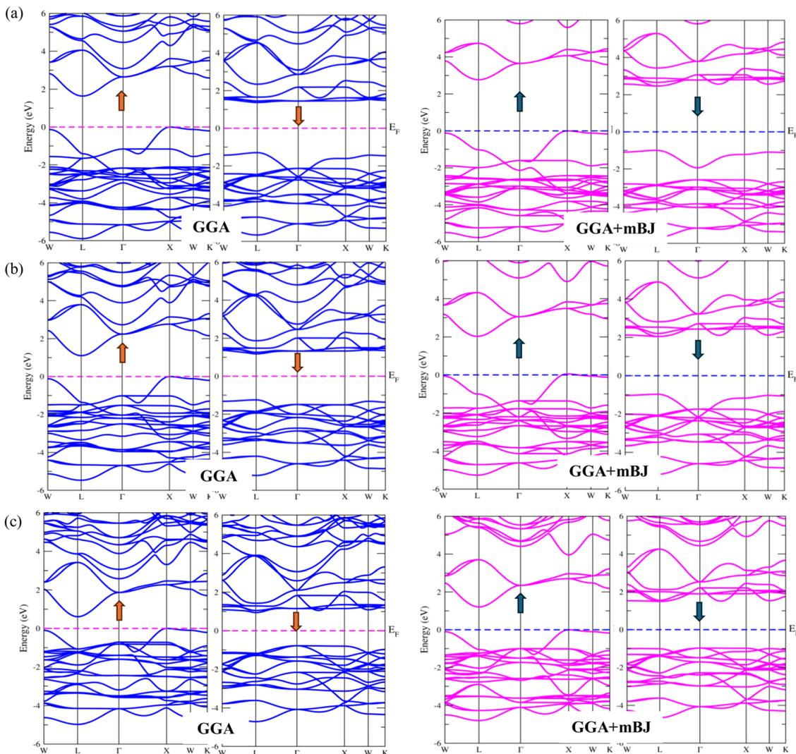
Fig. 6 DFT executed spin polarised band structure of (a)  $K_2GeMnCl_6$ , (b)  $K_2GeMnBr_6$ , and (c)  $K_2GeMnI_6$  halide perovskites calculated via GGA and GGA+mBJ approximations. The upward arrow represents the spin-up channel, while the downward arrow signifies the spin-down channel.
