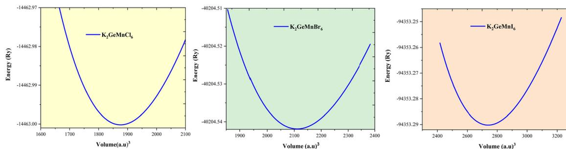
Fig. 1 Variation in total energy against unit cell volume for  $K_2GeMnX_6$  ( $X = Cl, Br, I$ ) determined via the GGA-PBE functional scheme.
