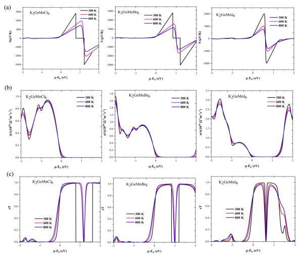
Fig. 12 Thermoelectric plots of (a) Seebeck coefficient (S), (b) electrical conductivity ( $\sigma/t$ ), and (c) figure of merit (zT) against chemical potential at different temperatures (300 K, 600 K, 800 K) for K<sub>2</sub>GeMnX<sub>6</sub> (X = Cl, Br, I) halide perovskites.
