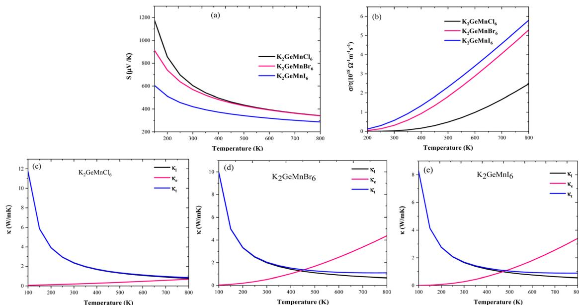
Fig. 11 Temperature variations for (a) Seebeck coefficient, (b) electrical conductivity, and (c)–(e) lattice, electronic and total thermal conductivity of  $\text{K}_2\text{GeMnX}_6$  halide perovskites.
