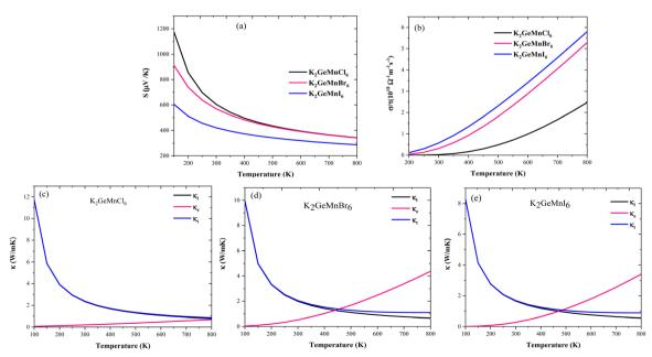
Fig. 11 Temperature variations for (a) Seebeck coefficient, (b) electrical conductivity, and (c)-(e) lattice, electronic and total thermal conductivity of K<sub>2</sub>GeMnX<sub>6</sub> halide perovskites
