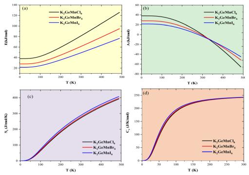
Fig. 5 Thermodynamic vibrational functions for  $K_2$ GeMn $X_6$  halide perovskites: (a) vibrational internal energy (*E*), (b) vibrational Helmholtz free energy (*A*), (c) vibrational entropy ( $S_v$ ) and (d) specific heat ( $C_v$ ) against a selected range of temperature.
