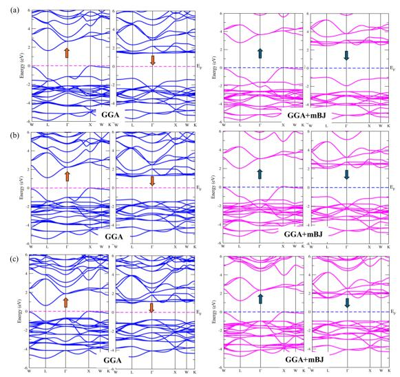
Fig. 6 DFT executed spin polarised band structure of (a)  $K_2$ GeMnCl<sub>6</sub>, (b)  $K_2$ GeMnBr<sub>6</sub>, and (c)  $K_2$ GeMnI<sub>6</sub> halide perovskites calculated *via* GGA and GGA+mBJ approximations. The upward arrow represents the spin-up channel, while the downward arrow signifies the spin-down channel.
