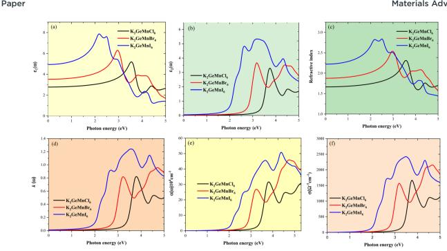
Fig. 10 The computed (a) real part of dielectric  $(\varepsilon_1(\omega))$ , (b) imaginary part of dielectric  $(\varepsilon_2(\omega))$ , (c) refractive index  $(n(\omega))$ , (d) extinction coefficient  $(k(\omega))$ , (e) absorption coefficient ( $\alpha(\omega)$ ) and (f) photoconductivity ( $\sigma$ ) for K<sub>2</sub>GeMnX<sub>6</sub> (X = Cl, Br, I) halide perovskites
