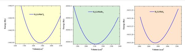
Fig. 1 Variation in total energy against unit cell volume for K<sub>2</sub>GeMnX<sub>6</sub> (X = Cl, Br, I) determined via the GGA-PBE functional scheme
