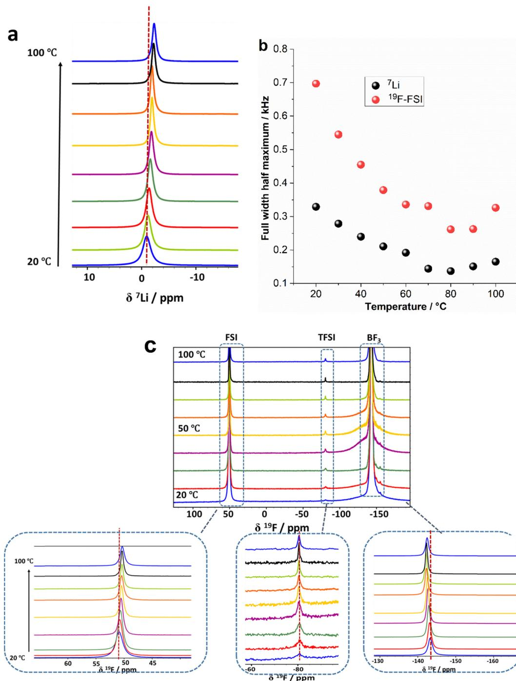
Fig. 6 (a) Static <sup>7</sup>Li NMR spectra of 90 vol% A/10 vol% NPs during first heating scan at different temperatures, (b) static <sup>7</sup>Li and <sup>19</sup>F linewidth of 90 vol% A/10 vol% NPs. (c) Static <sup>19</sup>F NMR spectra with heating.
