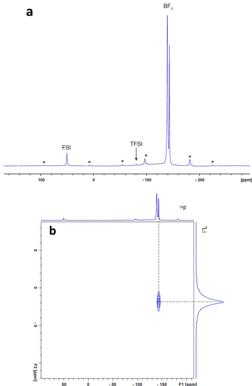
Fig. 7 High-field solid-state MAS NMR spectra obtained from the 90 vol% A/10 vol% NPs (a)  $^{19}\text{F}$  spectrum, (b)  $^{19}\text{F}$ - $^7\text{Li}$  HETCOR spectrum. \* indicates spinning side bands.
