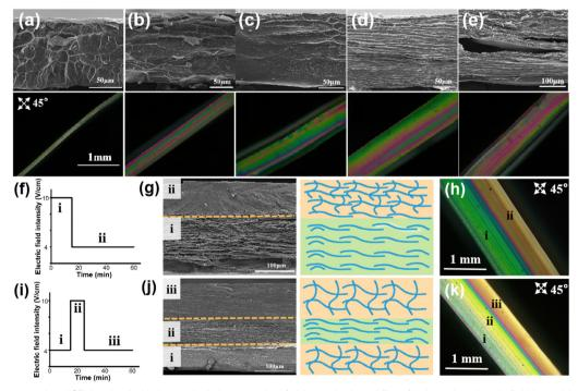
Fig. 3 (a)–(e) Cross-sectional SEM and polarization optical photographs of chitosan hydrogel films fabricated at electric field intensities of 2, 4, 6, 8, and  $10 \text{ V cm}^{-1}$ . The (f) two-step and (i) three-step electrical signal programs used to build E-CS with hierarchical structures. (g) and (j) Cross-sectional SEM images and schematics of the microstructures and (h) and (k) polarization optical photographs of the resultant bi- and tri-layer E-CS, respectively.
