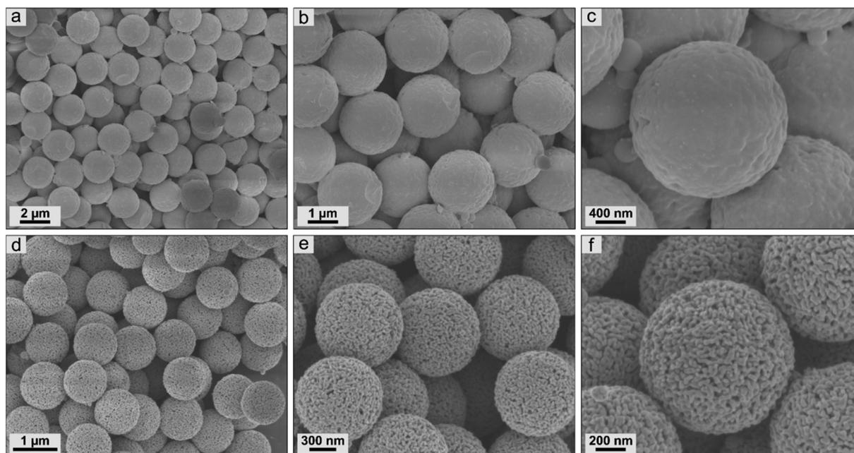
Fig. 5 Scanning electron micrographs of ceramic particles resulting from PS-ox@Fc-2 precursors by synthesis in (a)–(c) nitrogen and (d)–(f) synthetic air.
