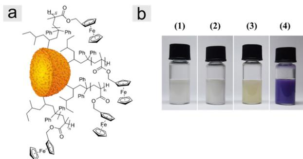
**Fig. 1** (a) Graphical representation of the structure of PSDVB@PFMMA functionalized particles and (b) images of *Preussmann* test results with PS-oxirane01 before and after epoxidation of PSDVB: (1) PSDVB particles in ethanol, (2) PSDVB particles and NBP in ethanol showing no reaction of PSDVB with the *Preussmann* reagent, (3) PS-oxirane particles in ethanol and (4) PS-oxirane particles after reaction with NBP in ethanol showing the positive *Preussmann* test.
