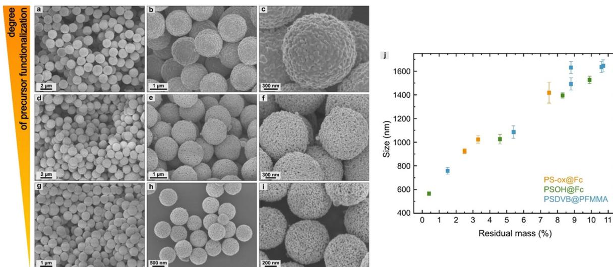
Fig. 9 (a)–(i) Scanning electron micrographs of ceramic particles based on PSDVB@PFMMA precursor with different degrees of functionalization: (a)–(c) PSDVB@PFMMA-3 (residual mass of 1.5%), (d)–(f) PSDVB@PFMMA-4 (residual mass of 8.8%), (g)–(i) PSDVB@PFMMA-2 (residual mass of 10.7%). (j) Overview of resulting particle sizes dependent on the residual mass and the different types of precursors.
