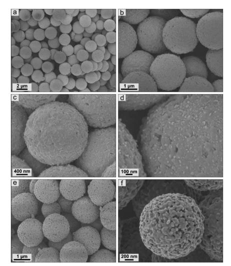
Fig. 6 Scanning electron micrographs of ceramic particles resulting from PSDVB@PFMMA-1 precursors by synthesis in (a)-(d) nitrogen and (e) and (f) synthetic air.
