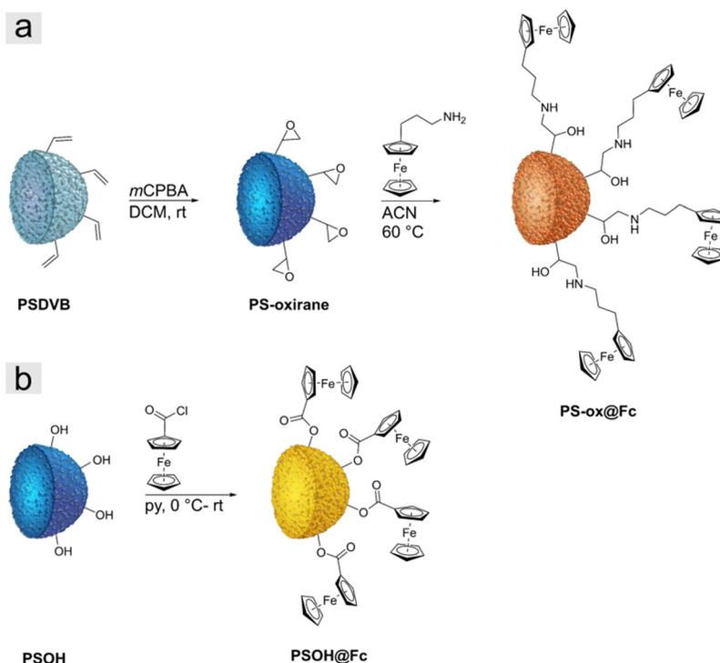
**Fig. 2** Graphical representation of the synthesis of (a) PS-ox@Fc particles starting from PSDVB particles by double bond epoxidation with *mCPBA* and ring-opening reaction with FcPA and (b) PSOH particles with ferrocene acid chloride leading to PSOH@Fc particles.
