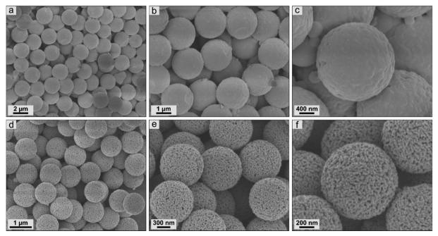
Scanning electron micrographs of ceramic particles resulting from PS-ox@Fc-2 precursors by synthesis in (a)-(c) nitrogen and (d)-(f) synthetic Fig. 5
