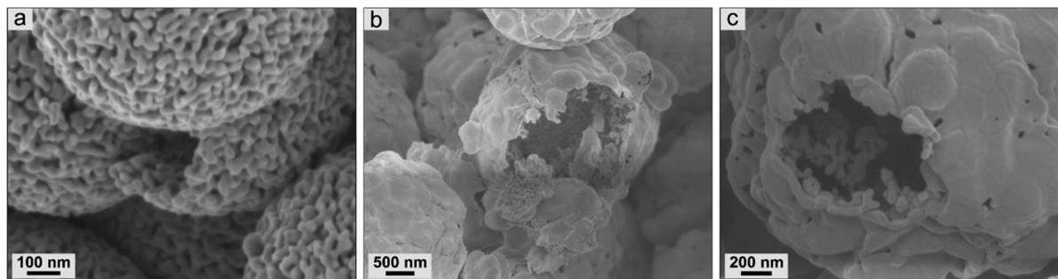
Fig. 10 Scanning electron micrographs proving a hollow structure by (a) broken ceramic particle based on PS-ox@Fc-2 and (b) and (c) broken particles based on PS-ox@Fc-4.
