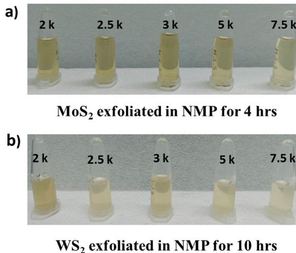
Fig. 2 (a) MoS<sub>2</sub> specimens exfoliated in NMP for 4 h. (b) WS<sub>2</sub> specimens exfoliated in NMP for 10 h. The specimens centrifuged at different rpm, viz. 2 krpm, 2.5 krpm, 3 krpm, 5 krpm and 7.5 krpm, respectively, are labelled as 2 k, 2.5 k, 3 k, 5 k and 7.5 k.
