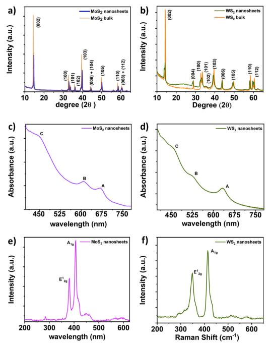
Fig. 3 X-Ray diffraction spectra of (a) MoS<sub>2</sub> and (b) WS<sub>2</sub> bulk and nanosheets; UV-vis spectra of (c) MoS<sub>2</sub> and (d) WS<sub>2</sub> nanosheets; Raman spectra of (e) MoS<sub>2</sub> and (f) WS<sub>2</sub> nanosheets.
