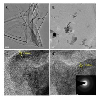
Fig. 5 TEM micrographs of few layer WS<sub>2</sub> nanosheets: (a) low magnification TEM micrograph (scale bar- $0.2 \mu m$ ); (b) low magnification TEM micrograph (scale bar-50 nm); (c) TEM micrograph of WS<sub>2</sub> nanosheets showing interlayer spacing (scale bar-2 nm); (d) TEM micrograph of WS<sub>2</sub> nanosheets showing lattice fringes, (scale bar-2 nm), inset shows the SAED pattern.
