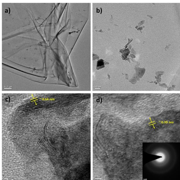
**Fig. 5** TEM micrographs of few layer WS<sub>2</sub> nanosheets: (a) low magnification TEM micrograph (scale bar-0.2 μm); (b) low magnification TEM micrograph (scale bar-50 nm); (c) TEM micrograph of WS<sub>2</sub> nanosheets showing interlayer spacing (scale bar-2 nm); (d) TEM micrograph of WS<sub>2</sub> nanosheets showing lattice fringes, (scale bar-2 nm), inset shows the SAED pattern.
