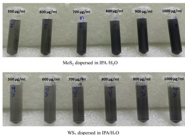
**Fig. 12** Different concentrations of exfoliated MoS<sub>2</sub> and WS<sub>2</sub> in IPA-H<sub>2</sub>O solvent after 6 h of exfoliation.
