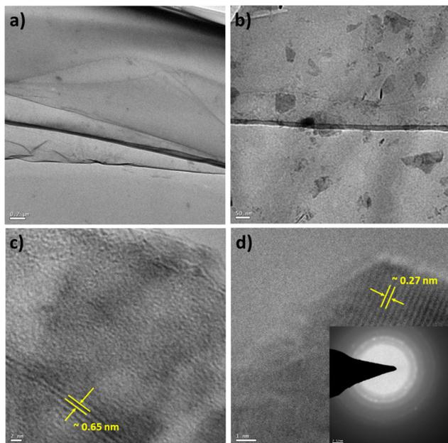
**Fig. 4** TEM micrographs of few-layer MoS<sub>2</sub> nanosheets: (a) low magnification TEM micrograph (scale bar-0.2 μm); (b) low magnification TEM micrograph (scale bar-50 nm); (c) TEM micrograph of MoS<sub>2</sub> nanosheets showing interlayer spacing (scale bar-2 nm); (d) TEM micrograph of MoS<sub>2</sub> nanosheets showing lattice fringes (scale bar-1 nm), with the inset showing the SAED pattern.
