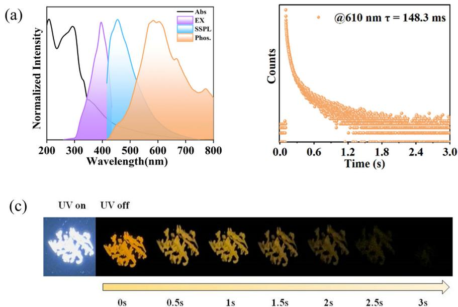
**Fig. 5** (a) Solid UV-vis absorption spectra, photoluminescence excitation spectrum at 395 nm, fluorescence emission, and phosphorescence emission spectra of **Form II** at room temperature. (b) Time-resolved emission decay profiles for **Form II** crystal at 454 and 610 nm excited by 395 nm. (c) The afterglow of **Form II** under 365 nm excitation.
