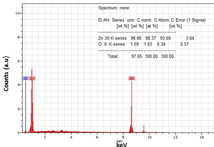
Fig. 7 EDS spectra of annealed ZnO samples.
