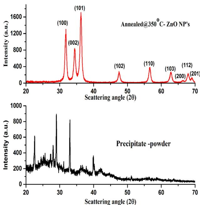
Fig. 2 XRD patterns of the as-dried (precipitate) sample and annealed ZnO NPs.
