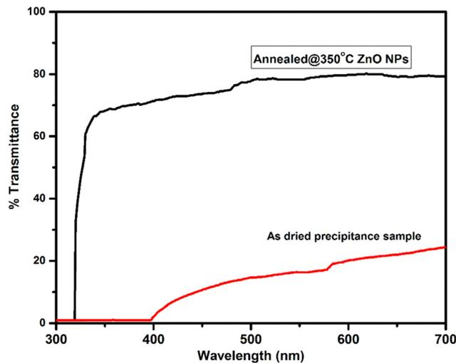
Fig. 4 Optical transmittance spectra of the ZnO NPs.
