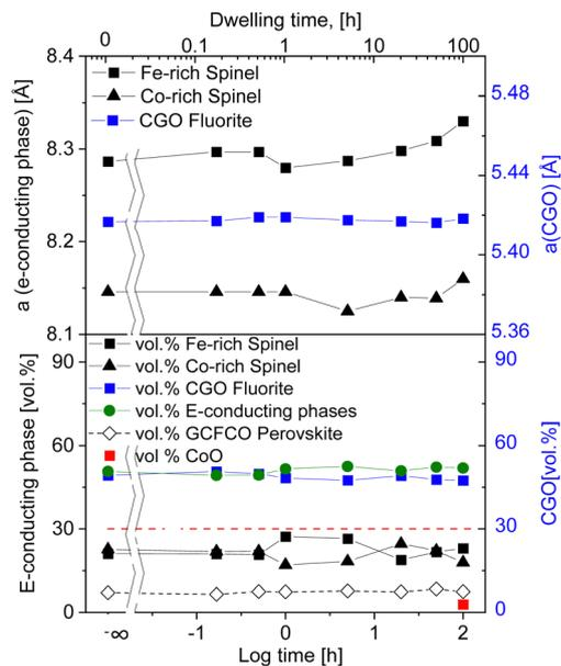
Fig. 2 Lattice parameter and volume fraction of observed phases in 60CGO20-FCO composites sintered at 1200 °C (solid lines are a guide to the eye).
