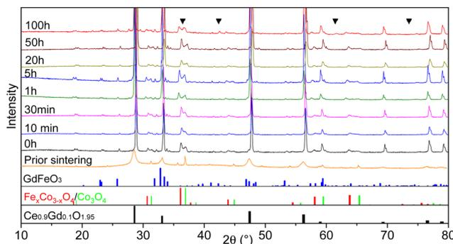
**Fig. 1** The XRD patterns of the 60CGO20–FCO composite sintered at 1200 °C with various dwell times, including an unsintered pellet. CoO rock salt phase peaks are marked as a triangle. At the bottom, reference reflections are shown for the perovskite in blue, spinel in red and green, and fluorite in black.
