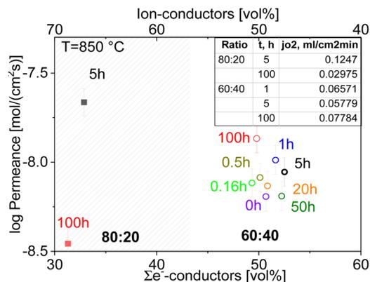
Fig. 15 Comparison of the final permeation performance of CGO20-FCO composite with ratio 60:40 and 80:20 sintered with various dwell times depending on the volume fraction of e<sup>-</sup>-conducting phases.
