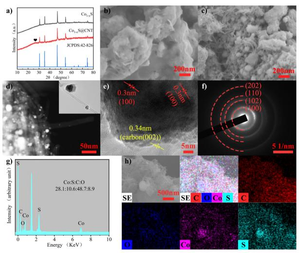
Fig. 1 (a) XRD pattern of  $Co_{1-x}S@CNTs$ . (b) SEM images of  $Co_{1-x}S$ . (c) SEM images of  $Co_{1-x}S@CNTs$ . (d) -(f) TEM images of  $Co_{1-x}S@CNTs$ . (g) EDS spectra of  $Co_{1-x}S@CNTs$ . (h) Corresponding EDS elemental mapping of Co, S, C, and O elements.
