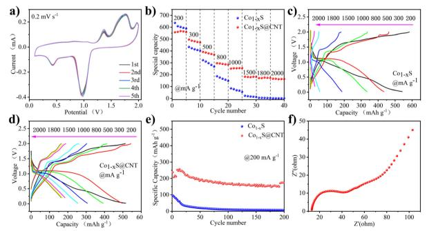
Fig. 3 (a) CV curves at 0.2 mV s<sup>-1</sup> of  $Co_{1-x}S@CNTs$ . (b) Rate performance of  $Co_{1-x}S@CNTs$ . (c) Charge-discharge profiles under different current densities of  $Co_{1-x}S$ . (d) Charge-discharge profiles under different current densities of  $Co_{1-x}S$ @CNTs. (e) Long-term cycling of  $Co_{1-x}S$  and  $Co_{1-x}$ S@CNT electrodes at 200 mA  $g^{-1}$ . (f) Nyquist plots for  $Co_{1-x}$ S@CNTs
