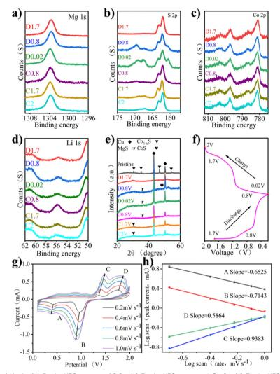
Fig. 4 (a) Ex situ XPS spectra of Mg 1s. (b) Ex situ XPS spectra of S 2p. (c) Ex situ XPS spectra of Co 2p. (d) Ex situ XPS spectra of Li 1s. (e) Ex situ XRD patterns of the  $Co_{1-x}S@CNT$  microspheres under different electrochemical stages. (f) Corresponding charge-discharge profiles. (g) Corresponding charge-discharge profiles. (h) CV curves at different scan rates of  $Co_{1-x}S@CNT$ . (i) logi-logv curves of  $Co_{1-x}S@CNT$ .
