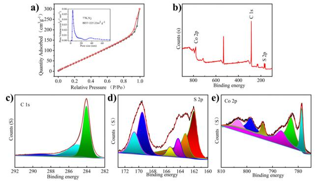
Fig. 2 (a)  $N_2$  adsorption—desorption isotherms, inset: corresponding pore size distribution. (b) Full XPS spectrum of  $Co_{1-x}S@CNT$ . (c) High resolution C 1s XPS spectrum. (d) High resolution S 2p XPS spectrum. (e) High resolution Co 2p XPS spectrum.
