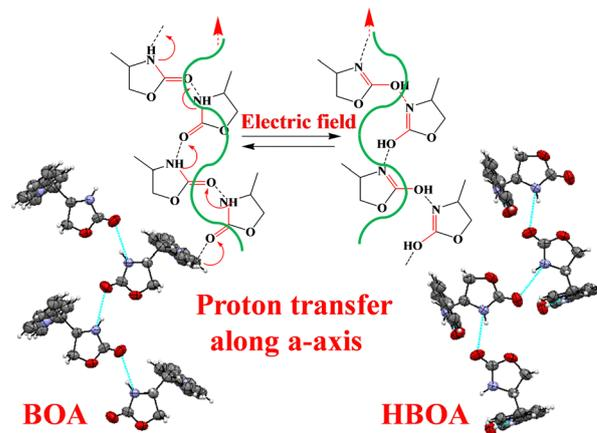
**Fig. 12** The crystal polarity can be inverted by proton transfer over a hydrogen bond and simultaneous interconversion of the single and double bonds, which are specified in red. The dotted lines indicate the proton transfer paths over the intermolecular  $\text{N-H}\cdots\text{O}$  hydrogen bonds. The thick arrow indicates the electric polarity of each hydrogen-bonded chain.
