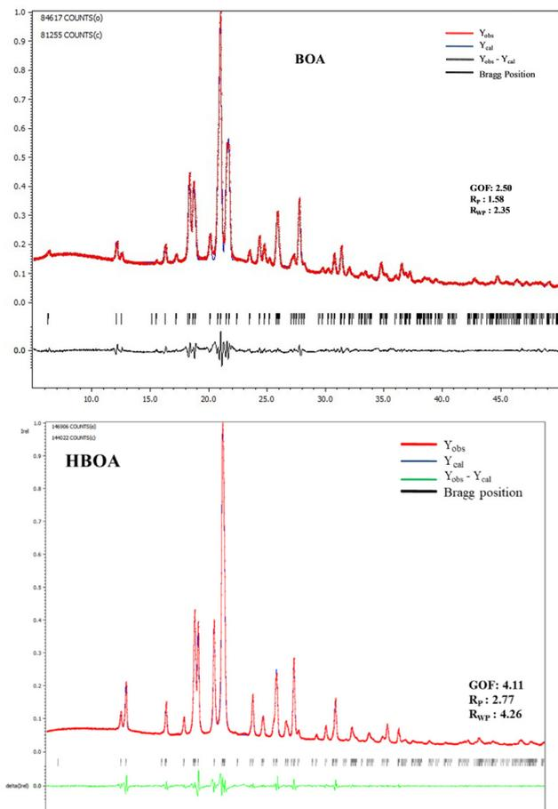
Fig. 3 PXRD pattern of the synthesized sample of BOA and HBOA.
