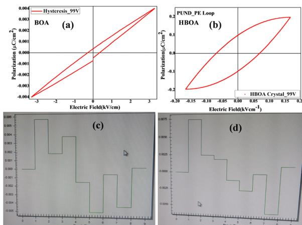
**Fig. 13** PUND data collected at an electric field of  $99 \text{ V cm}^{-1}$ , pulse width of 650 ms and pulse delay of 1000 ms for BOA and HBOA. (a) and (b) Hysteresis loop and switching polarization of BOA in the pellet. (c) and (d) Hysteresis loop and switching polarization of HBOA in the crystal.
