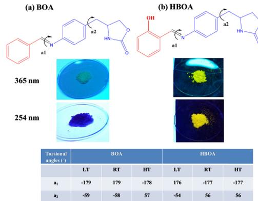
Fig. 1 Molecular structures of propeller shaped and solid emission of BOA and HBOA (as prepared) under UV light irradiation ( $\lambda = 254$  nm and 365 nm). Torsional angles are represented around the azomethine ( $-\text{C}=\text{N}-$ ) bond ( $a_1$ ) and methylene bond ( $-\text{CH}_2-$ ) ( $a_2$ ) attached to the chiral centre.
