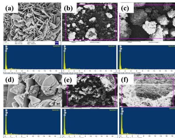
Fig. 8 (a) Crystalline, (b) unpoled and (c) poled SEM images of BOA. (d) Crystalline, (e) unpoled and (f) poled SEM images of HBOA. EDAX photographs (shown in blue colour) of BOA and HBOA are presented below their corresponding SEM images.
