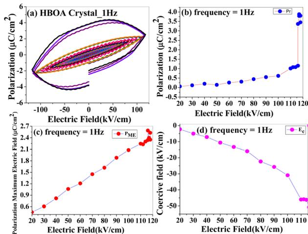
**Fig. 11** (a) Room temperature bipolar polarization hysteresis loops of the HBOA on the crystal at 1 Hz. (b)–(d) Correlation of remnant polarization ( $P_r$ ), polarization maximum electric field ( $P_{ME}$ ) and coercive field ( $E_c$ ) with an electric field at 1 Hz.
