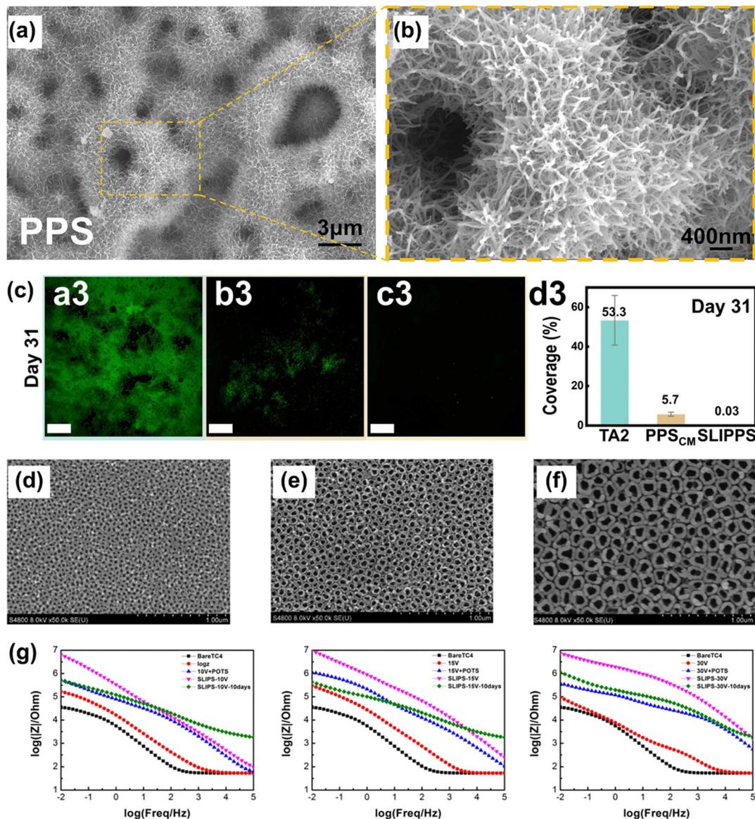
**Fig. 17** (a) and (b) SEM images of the surface morphologies of the PPS. (c) CLSM images of the Chlorella covering (reproduced from ref. 198 with permission from [Elsevier], copyright [2023]). (d)–(f) FE-SEM images of the TC4 anodic films formed at different voltages (10 V, 15 V, and 30 V). (g) Electrochemical impedance spectra of samples immersed in 3.5 wt% NaCl solution for 10 days (reproduced from ref. 199 with permission from [American Chemical Society], copyright [2019]).
