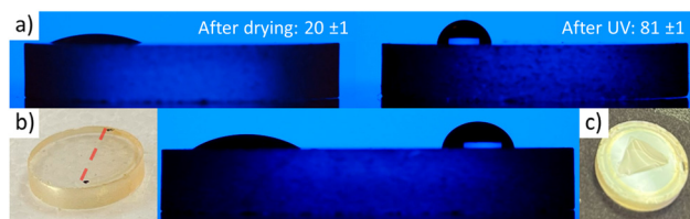
Fig. 5 (a) Example contact angle measurement of a thin film of 7-OH before (left) and after (right) 365 nm LED irradiation. (b) Example of the contact angle change in a single film of 9-OH, where half the film has been irradiated while the other half has been covered with a photomask. The red line in the picture (left) represents the location of the photomask, which gives rise to the change in the water droplet contact angle (right) on the same substrate. (c) Picture of how different photomasks can be used to control the surface wettability, herein a triangle shape photomask.
