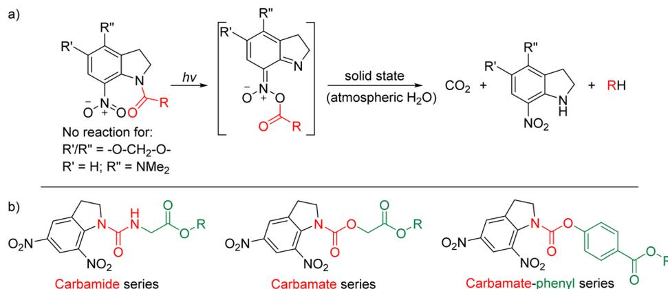
Fig. 1 (a) Schematic mechanism for the photocleavage of *o*-nitroanilide-based materials.<sup>22</sup> (b) The three series investigated in this study, where R = *tert*-butyl or H.
