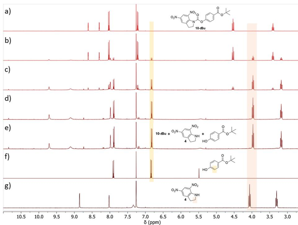
Fig. 4 Partial  $^1\text{H}$  NMR (400 MHz,  $\text{CDCl}_3$ ) spectra of (a)–(e) **10-tBu** after irradiation for 0, 1, 5, 15, and 30 min by  $2 \times 365$  nm LEDs ( $161 \text{ mW cm}^{-2}$  each); (f) *tert*-butyl 4-hydroxybenzoate; and (g) **4**. The shaded areas across the spectra highlight the change in some key signal peaks of the proposed photoproduct.
