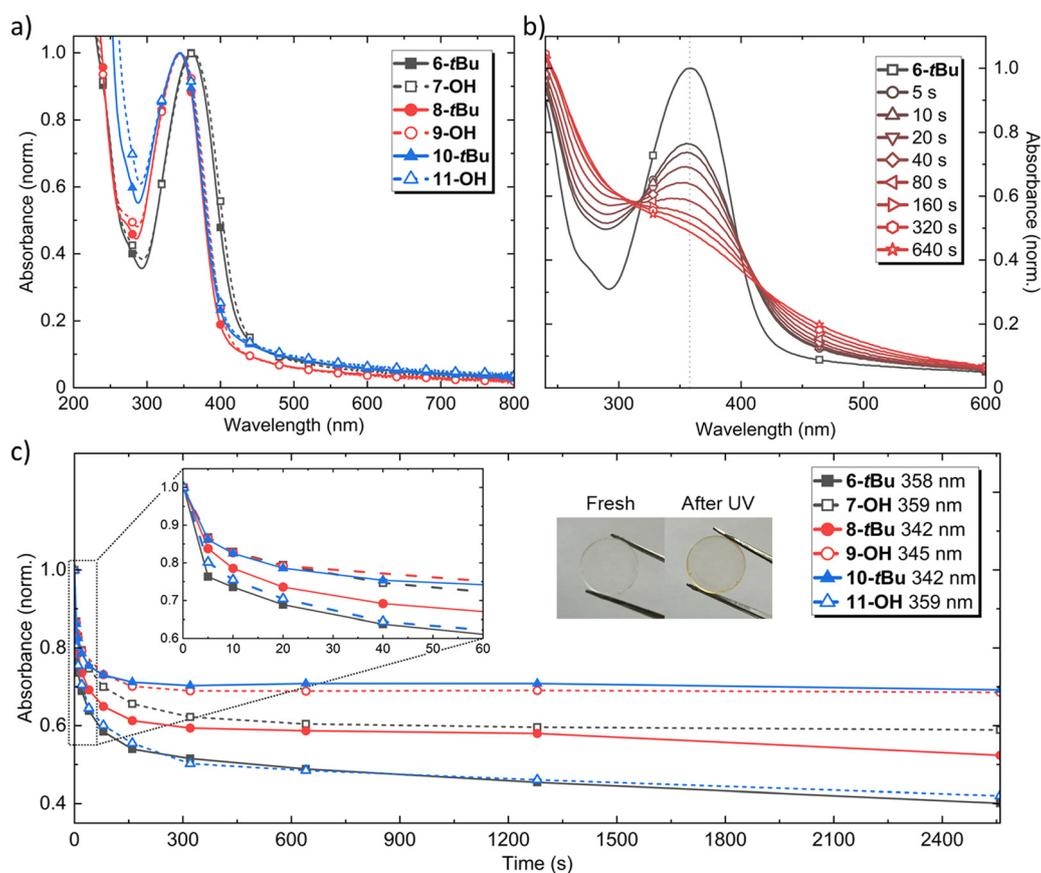
Fig. 3 (a) Neat film absorption of each of the materials. (b) Change in the UV-vis spectrum of **6-tBu** upon irradiation by a 365 nm LED. (c) Change in the peak absorption of each material upon 365 nm LED irradiation. Insert: Picture of a neat film of **6-tBu** before (left) and after (right) the irradiation experiment. The dashed vertical line in (b) represents the change plotted in (c). The LED power for all measurements was 161 mW cm<sup>-2</sup>.
