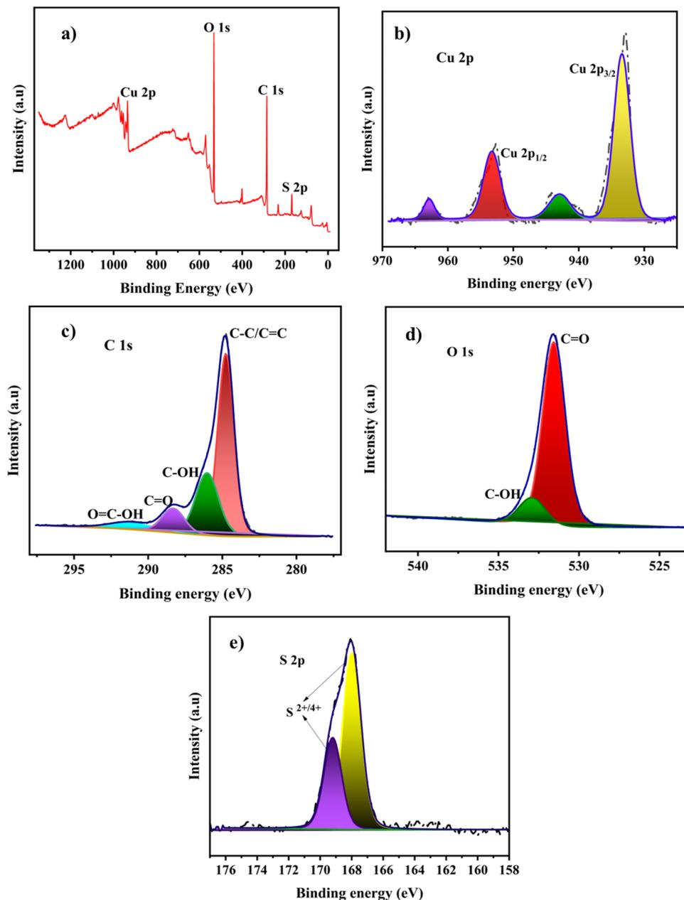
Fig. 2 (a) XPS survey spectrum of the Cu-BTC-MOF/PTA/CFP electrode, and core level spectra of (b) Cu 2p, (c) C 1s, (d) O 1s and (e) S 2p.
