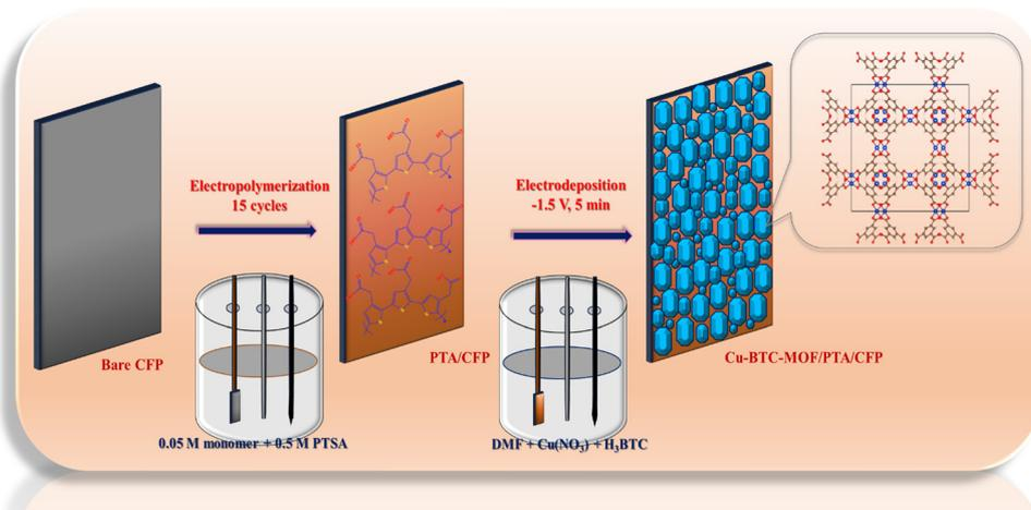
Scheme 1 Schematic illustration of the Cu-BTC-MOF/PTA/CFP electrode.
