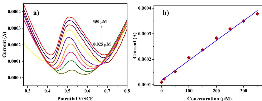
Fig. 7 (a) DPV graph of the Cu-BTC-MOF/PTA/CFP electrode in 0.2 M PBS (pH 7) at a sweep speed of  $0.05 \text{ V s}^{-1}$  with increasing concentration of RL. (b) The linear correlation between the concentration and anodic current intensity of RL.
