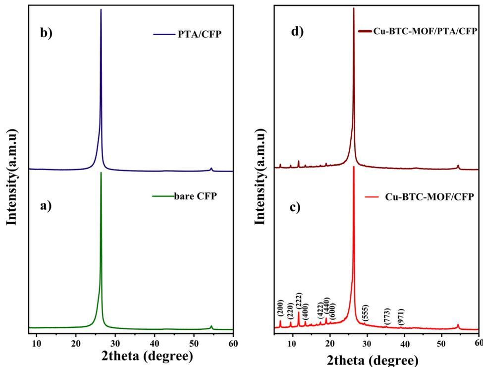
Fig. 1 X-Ray diffractogram of (a) bare CFP, (b) PTA/CFP, (c) Cu-BTC-MOF/CFP, and (d) Cu-BTC-MOF/PTA/CFP.
