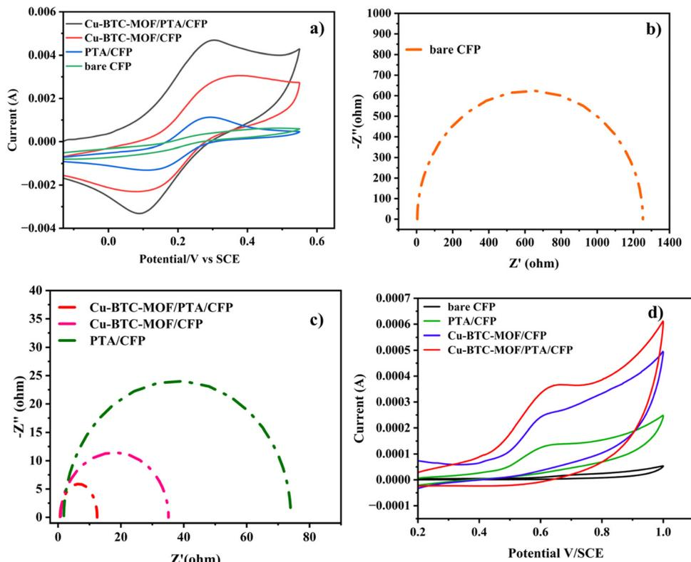
Fig. 4 (a) Cyclic voltammograms of the modified electrodes in 0.1 M KCl and 5 mM  $K_3[Fe(CN)_6]$  solution. (b) Nyquist plots of the bare CFP. (c) Nyquist plots of PTA/CFP, Cu-BTC-MOF/CFP, and Cu-BTC-MOF/PTA/CFP in the redox probe. (d) CVs of the bare CFP, PTA/CFP, Cu-BTC-MOF/CFP, and Cu-BTC-MOF/PTA/CFP in the presence of 120 nM RL in 0.2 M PBS (7) at a scanning speed of  $0.05 \text{ V s}^{-1}$ .
