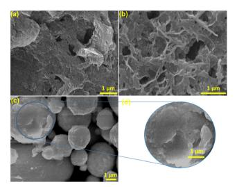
Fig. 2 SEM images of (a) g-C<sub>3</sub>N<sub>4</sub>, (b) PW<sub>11</sub>Ru-Mel, and (c) RuW/g-C<sub>3</sub>N<sub>4</sub>; (d) magnified image of RuW/g-C<sub>3</sub>N<sub>4</sub>.
