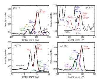
Fig. 5 The core level spectra of (a) C 1s, (b) Ru 3d, (c) O 1s and (d) W 4f of the RuW/g-C<sub>3</sub>N<sub>4</sub> composite
