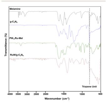
Fig. 1 FT-IR of Melamine, g-C<sub>3</sub>N<sub>4</sub>, PW<sub>11</sub>Ru-Mel, and RuW/g-C<sub>3</sub>N<sub>4</sub>.
