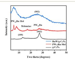
Fig. 4 XRD spectra of g-C<sub>3</sub>N<sub>4</sub>, PW<sub>11</sub>Ru-Mel, and RuW/g-C<sub>3</sub>N<sub>4</sub>.
