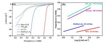
Fig. 6 (a) HER polarization curve and (b) the corresponding Tafel plots of PW<sub>11</sub>Ru, g-C<sub>3</sub>N<sub>4</sub>, and RuW/g-C<sub>3</sub>N<sub>4</sub> composites in comparison with Pt/C.
