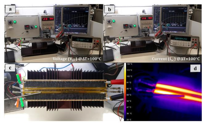
Fig. 7 GFRP-GTEG-device performance at  $\Delta T$ : 100 °C: (a) the generated open-circuit voltage ( $V_{OC}$ ) and, (b) the short-circuit current ( $I_{SC}$ ). (c) Thermoelectric power measurement set-up and (d) thermal image of the testing performance.
