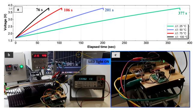
Fig. 8 (a) Diagram of the time required to charge the ALD-EH4295 utilizing the energy generated by the GFRP-GTEG to power up an LED at various  $\Delta T$ s. (b) and (c) The electronic board and the experimental setup containing the ALD-EH4295 employed at  $\Delta T$  = 100 °C to light up a green LED.
