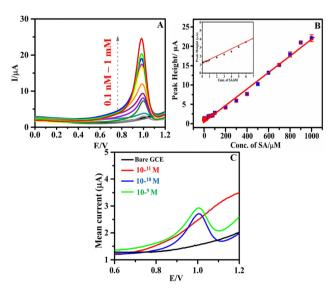
Fig. 4 (A) DPV responses of SA on h-BNNS/GCE from  $10^{-10}$  to  $10^{-3}$  M; (B) LDR obtained for the sensing of SA on the h-BNNS/GCE for the concentration range of  $10^{-10}$  to  $10^{-3}$  M (0.006 to 63 000 ppb) (inset: LDR fit obtained for the lower concentrations of SA (0.1-10 nM)); and (C) the DPV response of 0.006 ppb ( $10^{-10}$  M) SA on h-BNNS/GCE in 0.1 M PBS at the scan rate of 80 mV s<sup>-1</sup>
