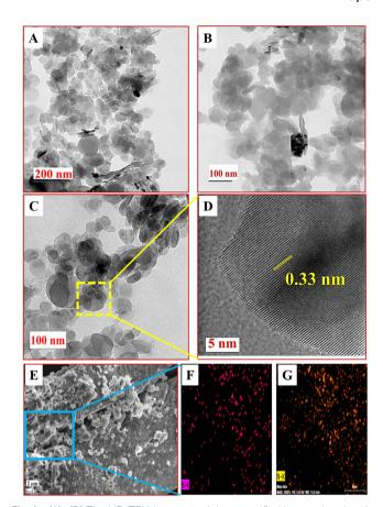
(A)-(D) The HR-TEM images and the magnified image showing the d-spacing of h-BNNS; (E) the SEM image of the h-BNNS; and (F) and (G) the SEM elemental mapping results of h-BNNS revealing the distribution of
