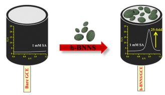
Scheme 2 The schematic shows the enhancement in the current response for SA in DPV on modification of the GCE with h-BNNS.
