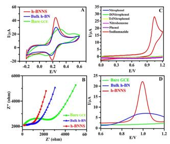
Fig. 3 (A) and (B) The CV and Nyquist diagrams of bare GCE, bulk h-BN/GCE, and h-BNNS/GCE in 5 mM [Fe(CN) $_6$ ]<sup>3-</sup>; (C) the CV response for 1 mM NP, DNP, TNP, PH, NB, PH, and SA on h-BNNS/GCE; and (D) the DPV response for 1 mM SA on GCE, bulk h-BN/GCE, and h-BNNS/GCE in 0.1 M PBS at the scan rate of 80 mV s<sup>-1</sup>.
