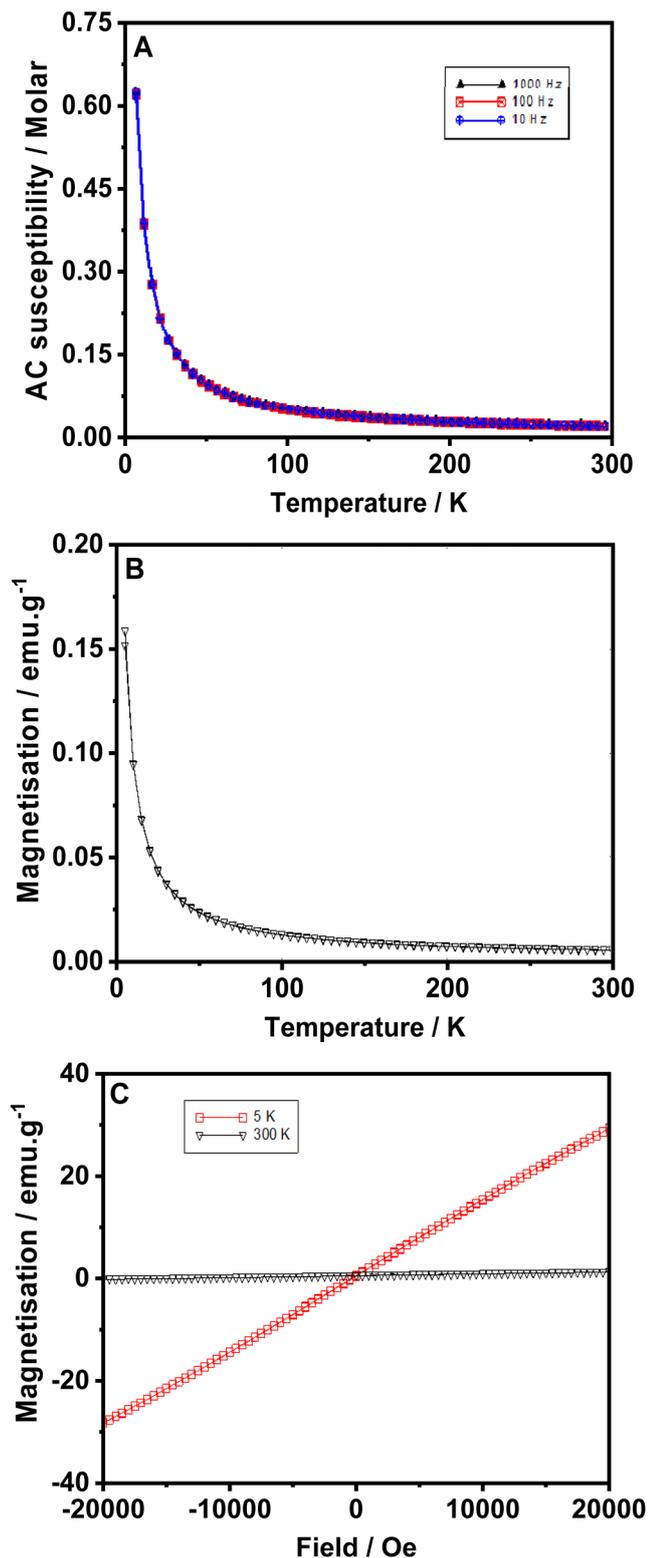
Fig. 9 (A) Temperature-dependence of the magnetic susceptibility of **1** at 10 Hz (blue), 100 Hz (red) and 1000 Hz (black). (B) Magnetization of **1** as a function of temperature at 100 Oe. (C) Plot of magnetization as a function of the magnetic field of **1** measured at 5 and 300 K.
