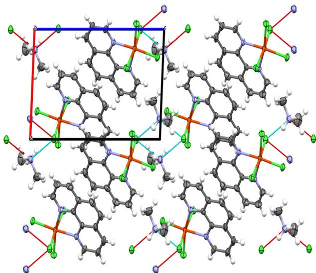
Fig. 3 Packing diagram of **1** along the *b*-axis. Carbon, nitrogen, hydrogen, iron and chlorine atoms are shown in dark grey, blue, white, dark orange and green, respectively, showing intermolecular (dashed lines) N–H...Cl hydrogen bonds.
