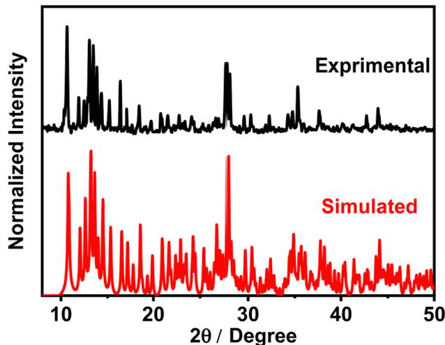
Fig. 1 Experimental (black line) and simulated (red line) X-ray diffraction patterns of (CH<sub>3</sub>)<sub>2</sub>NH<sub>2</sub>[Fe(phen)Cl<sub>4</sub>].
