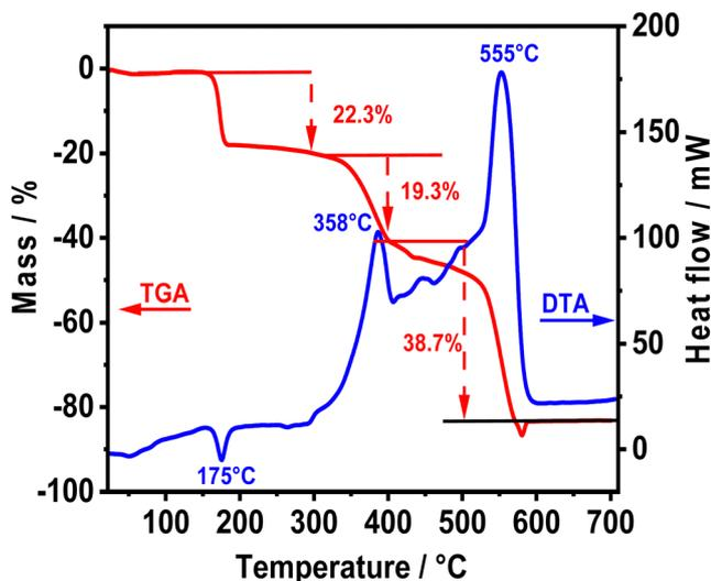
Fig. 8 TGA and DTA behaviours of complex **1**.
