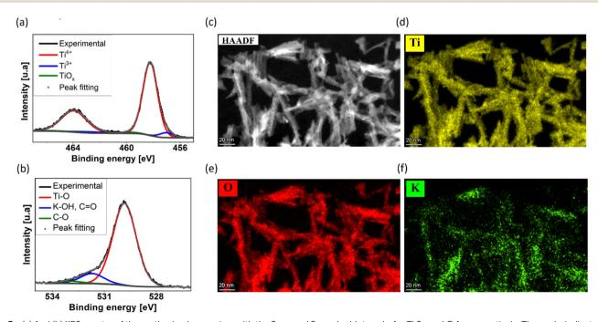
Fig. 3 (a) And (b) XPS spectra of the synthesized nanowires with the  $2p_{1/2}$  and  $2p_{3/2}$  doublet peaks for Ti 2p and O 1s, respectively. The peaks indicate the presence of Ti with different oxidation states. (c) STEM-HAADF image of a nanowire network. (d), (e) and (f) corresponding STEM-EDX elemental maps of nanowires for Ti-K, O-K, and K-K, respectively
