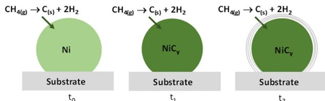
Fig. 8 Model of carbon diffusion into cubic nickel nanocrystal during  $\text{H}_2$ -Ar plasma exposure starting from  $\text{CH}_4$  hydrocarbon. Nickel carbide's carbon concentration increases leading, at supersaturation, to its demixing as an outer thin carbon graphitic shell (adapted from ref. 40).
