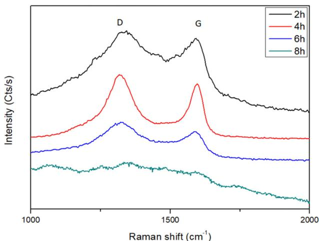
**Fig. 7** Raman spectra recorded on the  $\text{H}_2$ –Ar plasma-treated turbostratic disordered  $\alpha$ -hydroxide powder for different exposure times, highlighting the presence of almost disordered graphite.
