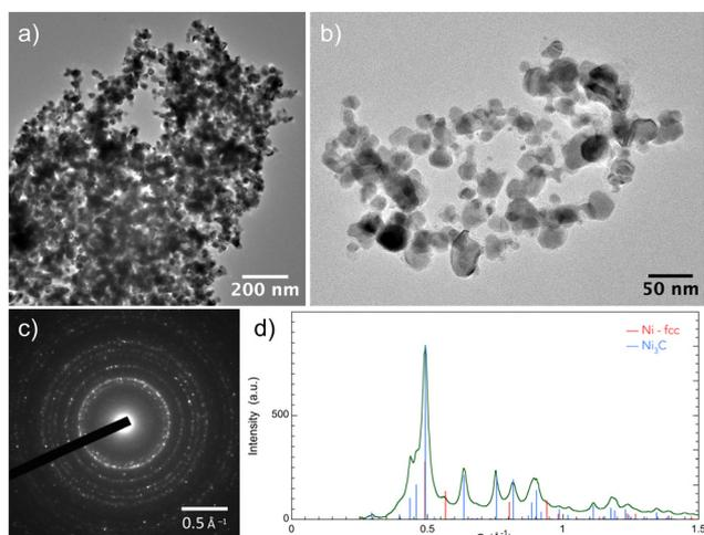
**Fig. 2** (a)–(b) TEM bright field image of an assembly of particles recovered after 2 h of H<sub>2</sub>-Ar plasma exposure of the turbostratic disordered  $\alpha$ -hydroxide powder. (c) Corresponding SAED pattern. (d) Radial intensity profile related to the SAED, showing the presence of Ni<sub>3</sub>C (ICDD No. 98-001-7005) as the major phase and Ni-fcc (ICDD No. 98-005-2265) as the minor phase.
