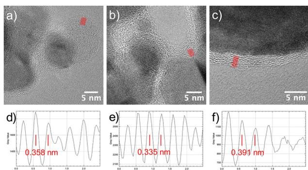
**Fig. 5** (a)–(c) HRTEM images evidencing the presence of graphitic carbon layer on  $\text{Ni}_3\text{C}$  and  $\text{NiC}_y$  particles recovered after 2 h of  $\text{H}_2$ –Ar plasma exposure of the turbostratic disordered  $\alpha$ -hydroxide powder. (d) and (f) Intensity profiles corresponding to the red lines in (a)–(c); the deduced mean interplanar distances are indicated.
