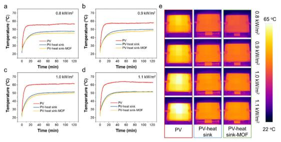
Fig. 4 The temperature change of PV panels with different device configurations at different sunlight intensities. (a)-(d): 0.8, 0.9, 1.0, and 1.1 kW m<sup>-2</sup>, respectively. (e) IR images of the PV panel under different conditions.
