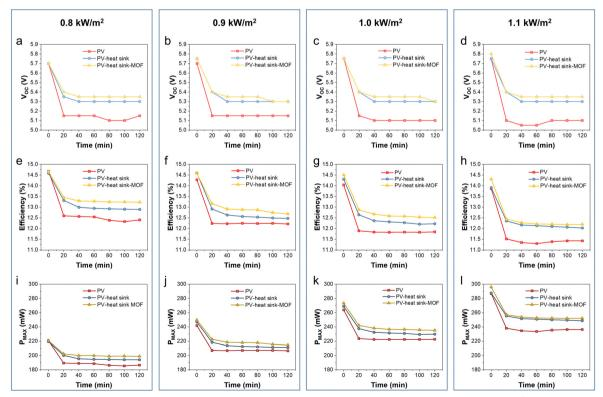
Fig. 6 The PV characteristics under different device configurations and at different sunlight intensities. (a), (e) and (i):  $0.8 \text{ kW m}^{-2}$ . (b), (f) and (j):  $0.9 \text{ kW m}^{-2}$ . (c), (g) and (k):  $1.0 \text{ kW m}^{-2}$ . (d), (h) and (l):  $1.1 \text{ kW m}^{-2}$ .
