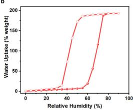
Fig. 1 (a) Crystal structure of Super-adsorbent Cr-soc-MOF-1. (b) Water sorption isotherm at 298 K for activated Cr-soc-MOF-1.
