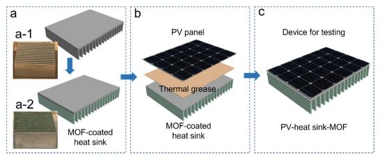
Fig. 2 Schematic of device assembly processes. (a) the MOF coating process; (a-1) photo of the heat fins before spray coating; (a-2) photo of the heat fins after spray coating with Cr-soc-MOF-1. (b) The device assembling process. (c) The as-assembled devices for testing.
