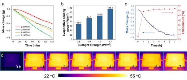
Fig. 5 The cooling performance of the Cr-soc-MOF-1-coated heat sink at different sunlight intensities. (a) The mass change of the MOF during the test. (b) The calculated evaporative cooling power was contributed by the evaporation of water from the MOF. (c) The mass change of the MOF and the temperature change of the PV panel in a prolonged 7-hour cooling test. (d) The IR images of the PV panel at different time nodes.
