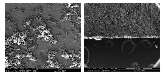
Top-view SEM images of the Cr-soc-MOF-1 particles as-synthesized (left) and after the spray coating process on the heat fins (right)
