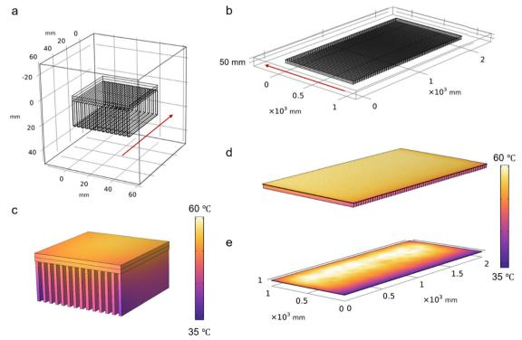
Fig. 7 COMSOL simulation of PV panel cooling effects at different dimensions. (a) and (b) Model and physical field of small-scale (4.5 × 4.5 cm²) and large-scale  $(1 \times 2 \text{ m}^2)$  devices, respectively, and the red arrows indicate the wind field directions. (c)–(e) Simulated temperature profile of small-scale and large-scale prototypes, and the large-scale pristine PV panel without cooling components.
