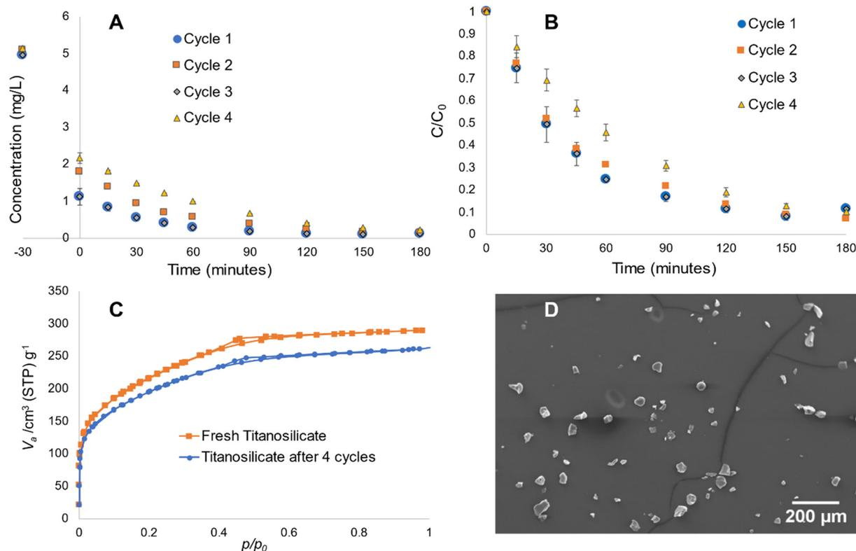
Fig. 8 Recyclability experiments on Rh B degradation with sample S as photocatalyst, over four cycles. (A) Concentration vs. time, (B) Normalized results ( $C/C_0$ ) vs. time, (C) comparative nitrogen adsorption–desorption isotherms for fresh and used titanosilicate and (D) SEM of used titanosilicate, showing non-fused/broken microspheres.
