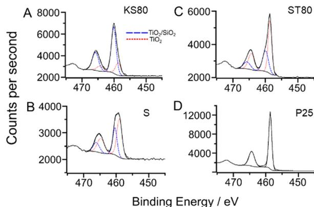
**Fig. 5** Fitted high resolution Ti 2p X-ray photoelectron scans of: A-sample KS80, B-sample S, C-sample ST80 and D-P25  $\text{TiO}_2$  standard. Fitted environments for KS80, S and ST80 were the same as those in our previous paper,<sup>29</sup> with a doublet separation of 5.72 eV. Samples KS80, S and ST80 exhibited differing ratios of  $\text{TiO}_2$  to  $\text{TiO}_2/\text{SiO}_2$  components, as listed in Table 2.
