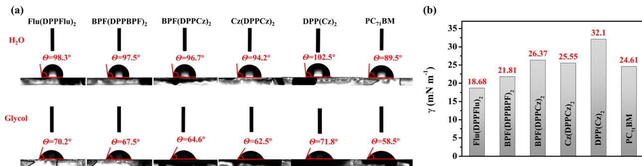
Fig. 9 (a) Contact angle images of water and ethylene glycol droplets for **Flu(DPPFlu)<sub>2</sub>**, **BPF(DPPBPF)<sub>2</sub>**, **BPF(DPPCz)<sub>2</sub>**, **Cz(DPPCz)<sub>2</sub>**, **DPP(Cz)<sub>2</sub>** and **PC<sub>71</sub>BM** on ITO/glass substrates; (b) surface energy histogram of different photovoltaic materials.
