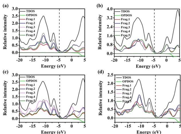
Fig. 3 The DOS curves of the designed molecules obtained with theoretical calculations: (a) **Flu(DPPFlu)<sub>2</sub>**, (b) **BPF(DPPBPF)<sub>2</sub>**, (c) **BPF(DPPCz)<sub>2</sub>**, and (d) **Cz(DPPCz)<sub>2</sub>**.
