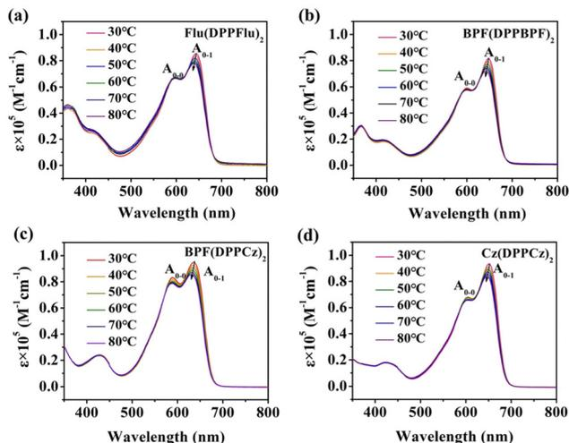
Fig. 6 Temperature-dependent absorption spectra of (a) **Flu(DPPFlu)<sub>2</sub>**, (b) **BPF(DPPBPF)<sub>2</sub>**, (c) **BPF(DPPCz)<sub>2</sub>**, and (d) **Cz(DPPCz)<sub>2</sub>** in dilute *o*-dichlorobenzene solutions at a temperature interval of 10 °C.
