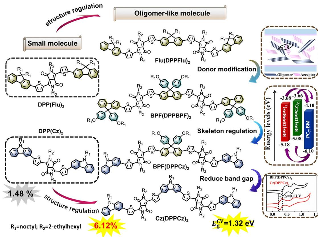
Scheme 1 Molecular design ideas and chemical structures of oligomer-like molecules Flu(DPPFlu)<sub>2</sub>, BPF(DPPBPF)<sub>2</sub>, BPF(DPPCz)<sub>2</sub>, and Cz(DPPCz)<sub>2</sub>.
