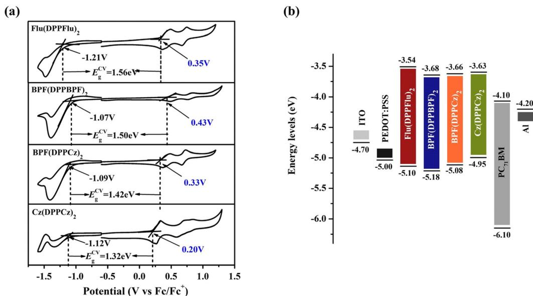
Fig. 7 Electrochemical cyclic voltammetry curves and energy levels: (a) CV curves of **Flu(DPPFlu)<sub>2</sub>**, **BPF(DPPBPF)<sub>2</sub>**, **BPF(DPPCz)<sub>2</sub>**, and **Cz(DPPCz)<sub>2</sub>** in 0.1 M Bu<sub>4</sub>NBF<sub>4</sub>/CH<sub>2</sub>Cl<sub>2</sub> solution at a scan rate of 100 mV s<sup>-1</sup> under nitrogen atmosphere; (b) energy level diagram of the four materials and PC<sub>71</sub>BM.
