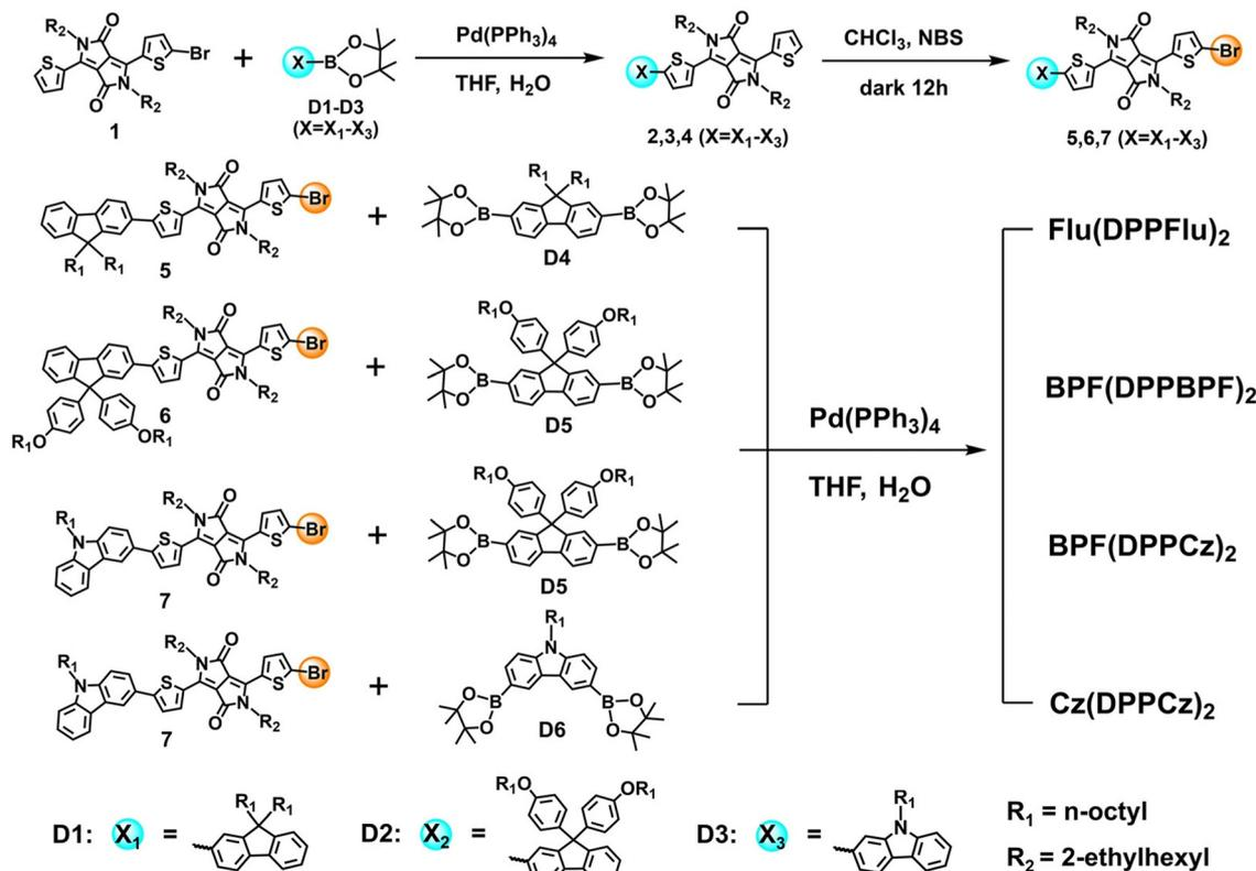
Scheme 2 Synthetic routes for the target compounds Flu(DPPFlu)<sub>2</sub>, BPF(DPPBPF)<sub>2</sub>, BPF(DPPCz)<sub>2</sub> and Cz(DPPCz)<sub>2</sub>.
