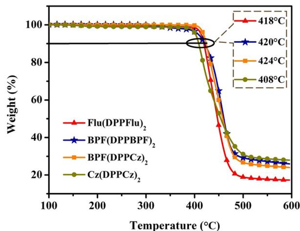
Fig. 1 TGA curves of compounds Flu(DPPFlu)<sub>2</sub>, BPF(DPPBPF)<sub>2</sub>, BPF(DPPCz)<sub>2</sub> and Cz(DPPCz)<sub>2</sub> at a heating rate of 10 °C min<sup>-1</sup> under nitrogen flow.
