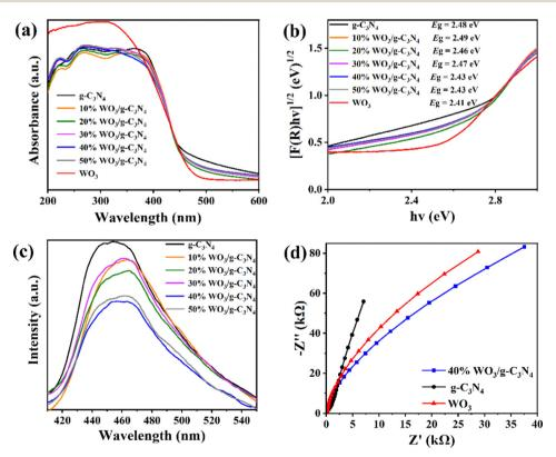
Fig. 4 (a) UV-vis DRS spectra, (b)  $E_q$  and (c) PL spectra of the g-C<sub>3</sub>N<sub>4</sub>, WO<sub>3</sub> and WO<sub>3</sub>/g-C<sub>3</sub>N<sub>4</sub> composites; (d) EIS of 40%WO<sub>3</sub>/g-C<sub>3</sub>N<sub>4</sub>, g-C<sub>3</sub>N<sub>4</sub> and WO<sub>3</sub>.
