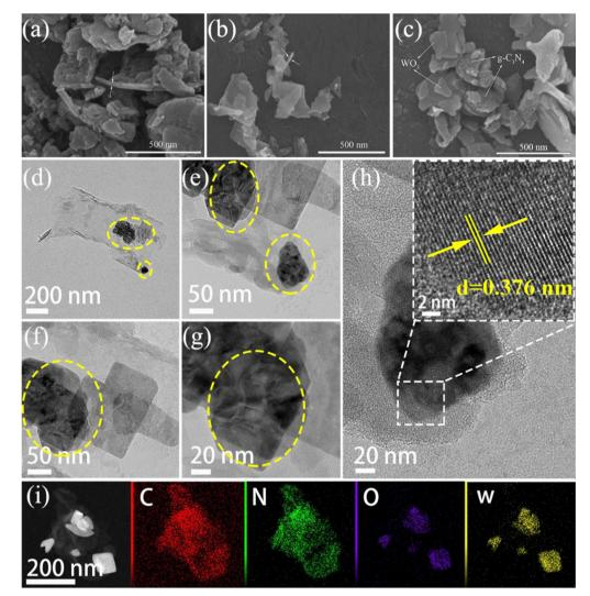
Fig. 3 SEM images of (a)  $g-C_3N_4$ , (b)  $WO_3$  and (c)  $40\%WO_3/g-C_3N_4$ ; (d)–(h) HRTEM images and (i) EDS mapping images of  $40\%WO_3/g$   $C_3N_4$ .
