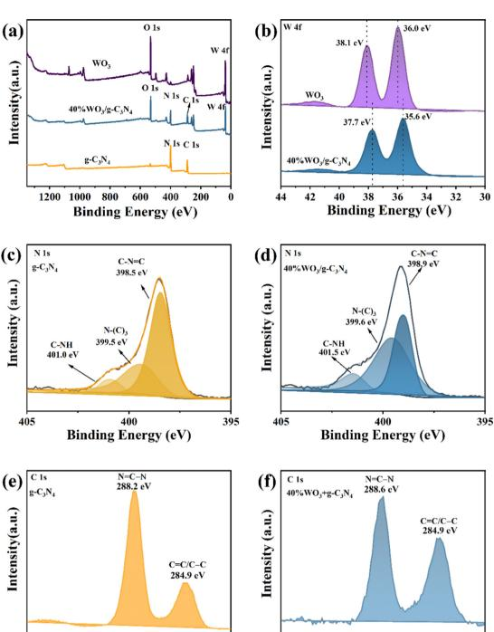
Fig. 2 (a) XPS survey spectra of  $q-C_xN_4$  and  $40\%WO_x/q-C_xN_4$ , (b) high-resolution W 4f spectra of  $WO_x$  and  $40\%WO_x/q-C_xN_4$ , (c) high-resolution N1s spectra of  $g-C_3N_4$ , (d) high-resolution N1s spectra of  $40\%WO_3/g-C_3N_4$ , (e) high-resolution C1s spectra of  $g-C_3N_4$  and (f) high-resolution C 1s spectra of 40%WO<sub>3</sub>/g-C<sub>3</sub>N<sub>4</sub>
