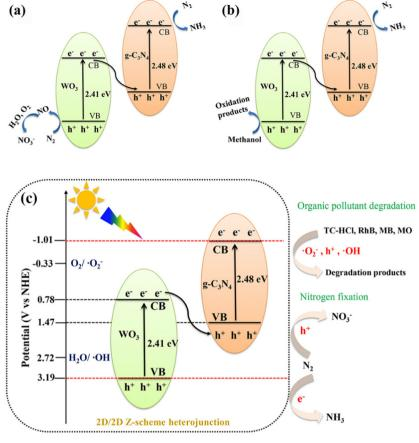
Fig. 9 The proposed photocatalytic nitrogen fixation mechanism of 40%WO<sub>3</sub>/q-C<sub>3</sub>N<sub>4</sub>: (a) Experiment 1 and (b) Experiment 2; and (c) the proposed photocatalytic mechanism of the 2D/2D Z-scheme WO<sub>3</sub>/g-C<sub>3</sub>N<sub>4</sub> heterojunctions in this work.
