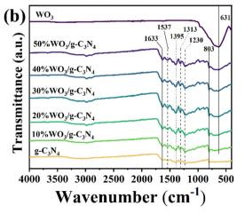
Fig. 1 (a) XRD and (b) FT-IR spectra of the  $g-C_3N_4$ ,  $WO_3$  and  $WO_3/g-C_3N_4$  composites
