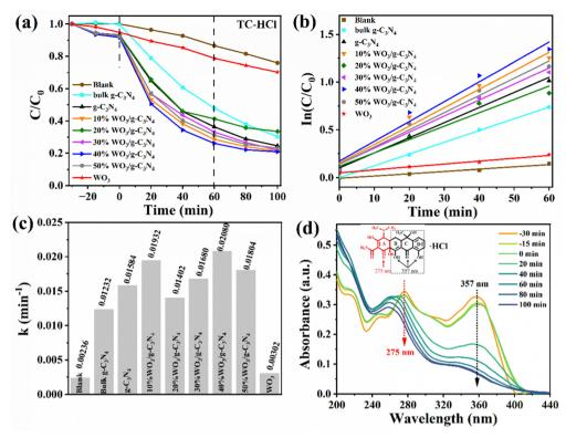
Fig. 5 (a) The photocatalytic degradation efficiency of TC-HCl by  $g-C_3N_4$ ,  $WO_3$  and  $WO_3/g-C_3N_4$  composites under visible light, (b) corresponding firstorder kinetic fitting curves and (c) corresponding UV-vis absorption spectra during the degradation of TC-HCl by 40%WO<sub>3</sub>/g-C<sub>3</sub>N<sub>4</sub>.
