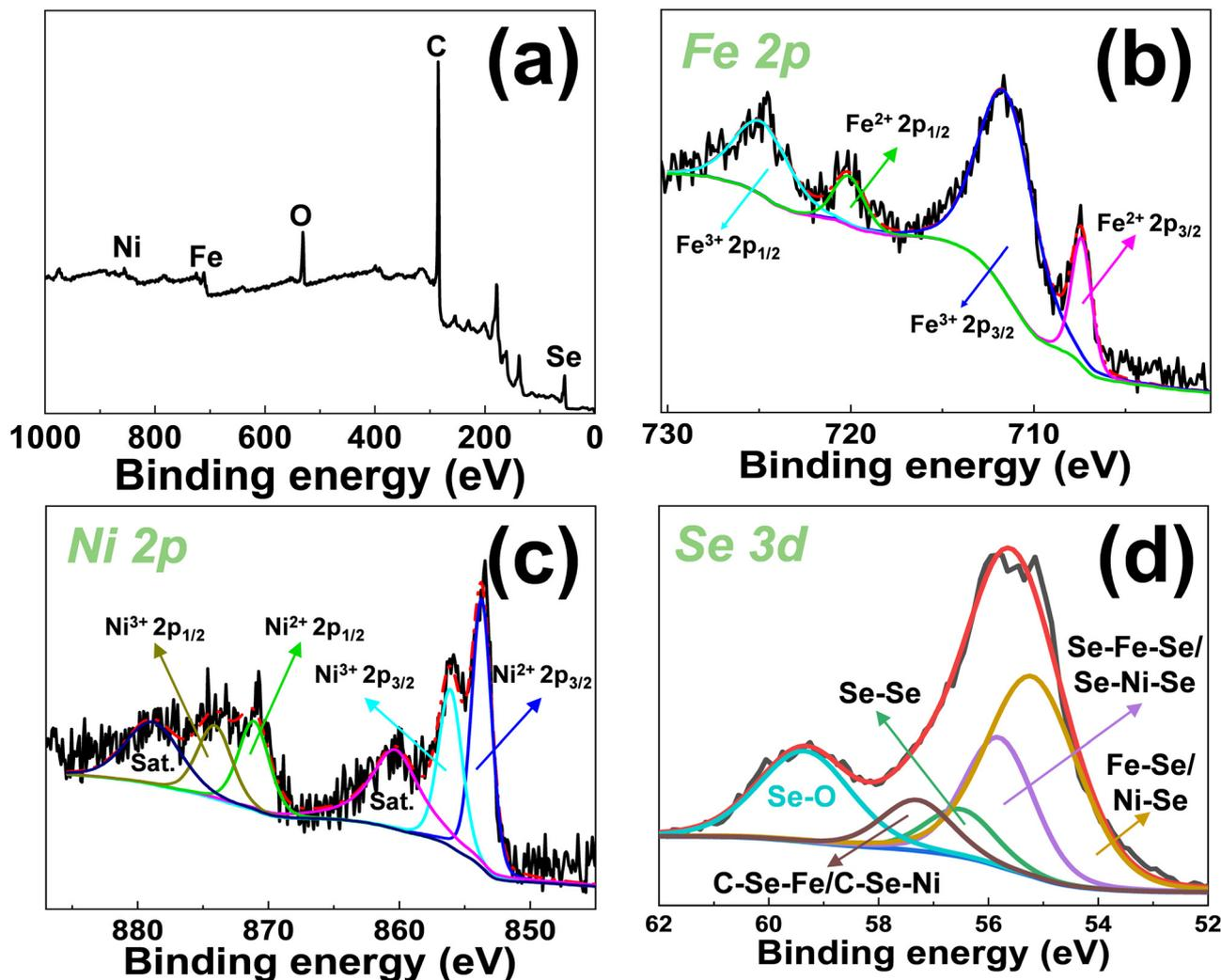
Fig. 4 (a) XPS spectrum of FeNiSe<sub>4</sub>@PG and its (b) Fe 2p, (c) Ni 2p, and (d) Se 3d spectra.
