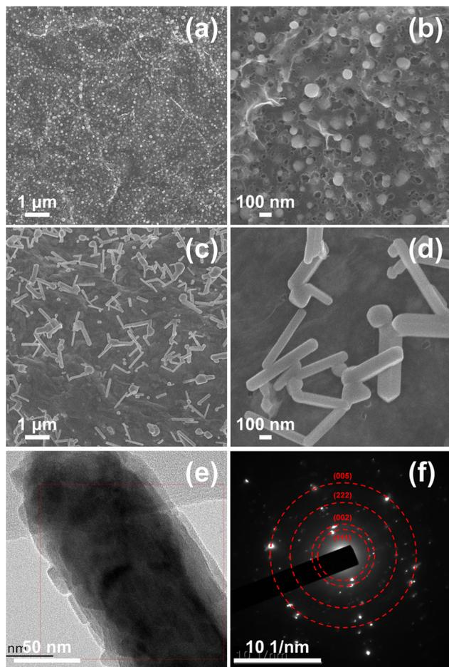
Fig. 2 SEM images of (a) and (b) FeNi@PG and (c) and (d) FeNiSe<sub>4</sub>@PG. (e) TEM image of FeNiSe<sub>4</sub>@PG and (f) corresponding SAED pattern.
