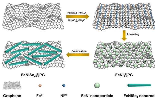
Fig. 1 Schematic diagram of the forming process of FeNiSe<sub>4</sub>@PG.
