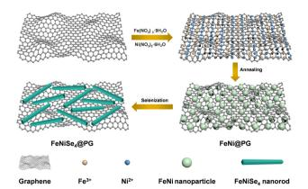
Fig. 1 Schematic diagram of the forming process of FeNiSe<sub>4</sub>@PG.
