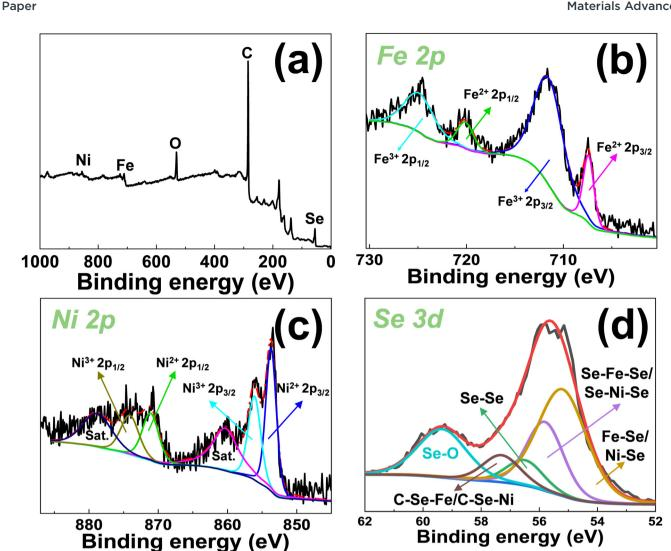
(a) XPS spectrum of FeNiSe₄@PG and its (b) Fe 2p, (c) Ni 2p, and (d) Se 3d spectra.
