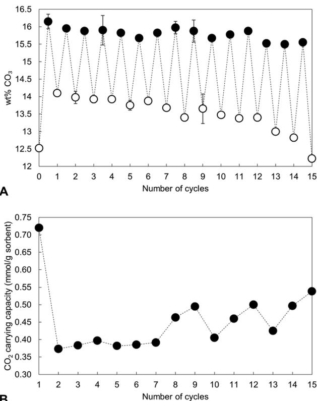
Fig. 4 (A) Measured carbonate content of the *x* = 2.5 apatite as-prepared and over 15 cycles at 500 °C. Filled markers represent samples heated in dry CO<sub>2</sub> whereas open markers denote samples heated in air. (B) The carrying capacity of the material over these cycles, defined as the quantity of CO<sub>2</sub> absorbed during each carbonation.
