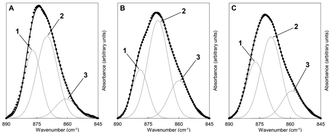
Fig. 7 Deconvolution of the carbonate  $\nu_2$  region of the FTIR spectra of the  $x = 2.5$  apatite (A) at the start of the first cycle *i.e.* the AP sample, (B) after carbonation and (C) after sorbent regeneration. Dashed lines correspond to the individual fitted peaks and the solid line the corresponding model spectra; the raw data is presented as isolated data points. The y-axis was plotted using an arbitrary scale.
