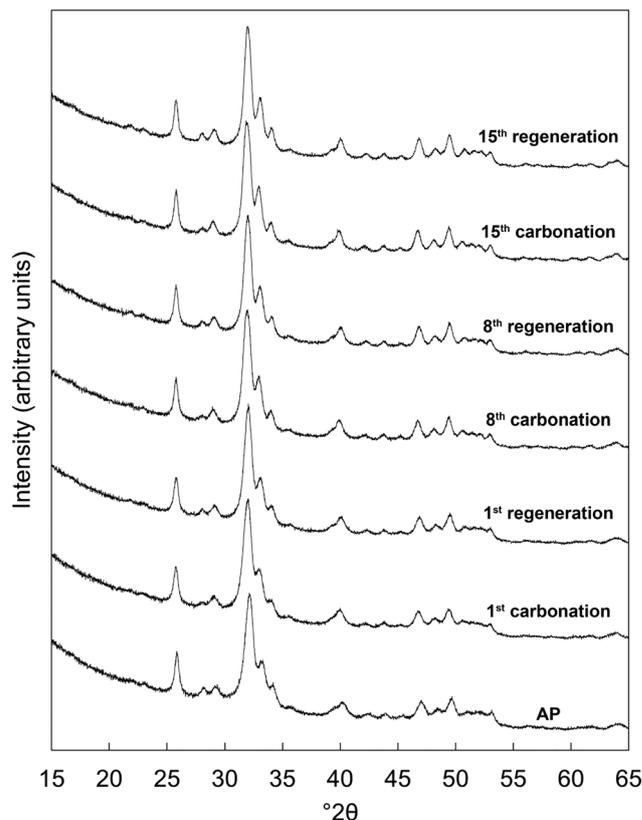
Fig. 3 Normalised ( $I_{\max} = 100$ ) X-ray diffraction patterns of the  $x = 2.5$  apatite as-prepared (AP) and at several intervals over 15 cycles at 500 °C in dry CO<sub>2</sub> and air respectively.
