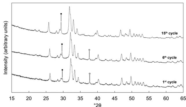
Fig. 5 Normalised ( $I_{\max} = 100$ ) XRD patterns of the *x* = 2.5 apatite after being cycled multiple times (1, 6 or 15 carbonation/regeneration steps at 500 °C), with the final decarbonation for each performed at 600 °C. Intense reflections corresponding to secondary phases of calcite and calcium oxide are marked using ● and ○ respectively.
