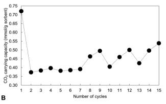
Fig. 4 (A) Measured carbonate content of the x=2.5 apatite as-prepared and over 15 cycles at 500 °C. Filled markers represent samples heated in dry  $CO_2$  whereas open markers denote samples heated in air. (B) The carrying capacity of the material over these cycles, defined as the quantity of  $CO_2$  absorbed during each carbonation.
