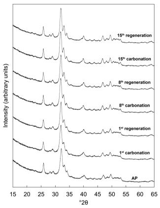
Fig. 3 Normalised ( $l_{\text{max}} = 100$ ) X-ray diffraction patterns of the x = 2.5 apatite as-prepared (AP) and at several intervals over 15 cycles at 500 °C in dry CO<sub>2</sub> and air respectively.
