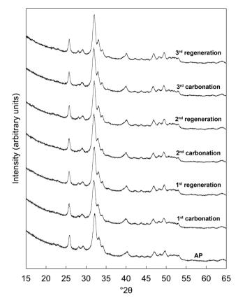
Fig. 1 Normalised ( $I_{max} = 100$ ) XRD patterns of the x = 2.5 apatite asprepared (AP) and over three carbonation-regeneration cycles at 500 °C in dry CO2 and air respectively
