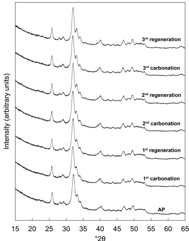
Fig. 1 Normalised ( $I_{\text{max}} = 100$ ) XRD patterns of the  $x = 2.5$  apatite as-prepared (AP) and over three carbonation–regeneration cycles at  $500\text{ }^\circ\text{C}$  in dry  $\text{CO}_2$  and air respectively.
