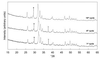
Fig. 5 Normalised ( $l_{\text{max}} = 100$ ) XRD patterns of the x = 2.5 apatite after being cycled multiple times (1, 6 or 15 carbonation/regeneration steps at 500 °C), with the final decarbonation for each performed at 600 °C. Intense reflections corresponding to secondary phases of calcite and calcium oxide are marked using  $\bullet$  and  $\bigcirc$  respectively.
