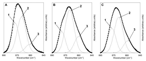
Fig. 7 Deconvolution of the carbonate  $\nu_2$  region of the FTIR spectra of the x = 2.5 apatite (A) at the start of the first cycle i.e. the AP sample, (B) after carbonation and (C) after sorbent regeneration. Dashed lines correspond to the individual fitted peaks and the solid line the corresponding model spectra; the raw data is presented as isolated data points. The y-axis was plotted using an arbitrary scale.
