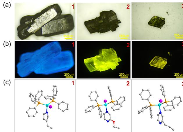
Fig. 2 Images of crystals of compounds 1–3 under white light (a) and 365 nm UV light (b), crystal structures of compounds 1–3 (c), different colors indicate various element atoms, light blue: Cu; yellow: P; grey: C; purple: I; deep blue: N; red: O.
