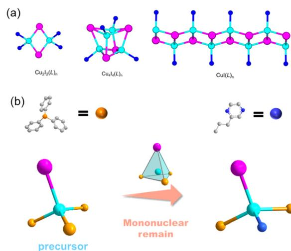
Fig. 1 (a) Typical structures of a rhomboid dimer 0D-Cu<sub>2</sub>I<sub>2</sub>(L)<sub>2</sub>, a cubane tetramer 0D-Cu<sub>4</sub>I<sub>4</sub>(L)<sub>4</sub>, and a staircase chain 1D-CuI(L). (b) Scheme of the bottom-up strategy for the mononuclear structure. Cyan balls: Cu, pink balls: I, blue balls: N-ligand, yellow balls: PPh<sub>3</sub>.
