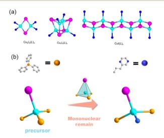
Fig. 1 (a) Typical structures of a rhomboid dimer OD-Cu<sub>2</sub>I<sub>2</sub>(L)<sub>4</sub>, a cubane tetramer 0D-Cu<sub>4</sub>I<sub>4</sub>(L)<sub>4</sub>, and a staircase chain 1D-CuI(L). (b) Scheme of the bottom-up strategy for the mononuclear structure. Cyan balls: Cu, pink balls: I, blue balls: N-ligand, yellow balls: PPh3.
