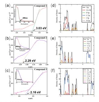
Fig. 3 (a)–(c) The optical diffuse reflectance spectra (inset) and the corresponding Tauc plots of compounds  $\mathbf{1}$ – $\mathbf{3}$ , respectively. (d)–(f) Calculated density of states of compounds  $\mathbf{1}$ – $\mathbf{3}$ . The total density of states (black); Cu 3d orbitals (red); P 3p orbitals (green); C 2p orbitals (blue); N 2p orbitals (brown); O 2p orbitals (dark pink).
