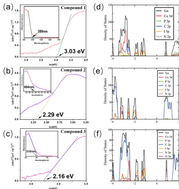
**Fig. 3** (a)–(c) The optical diffuse reflectance spectra (inset) and the corresponding Tauc plots of compounds **1–3**, respectively. (d)–(f) Calculated density of states of compounds **1–3**. The total density of states (black); Cu 3d orbitals (red); P 3p orbitals (green); C 2p orbitals (blue); N 2p orbitals (brown); O 2p orbitals (dark pink).
