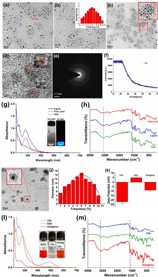
**Fig. 1** (a)–(d) High-resolution electron microscopy images of CDs. (e) SEAD pattern of only CDs. (f) XRD pattern of CDs. (g) UV-Vis spectra (h) FTIR spectra. (i) High-resolution electron microscopy images of DOX conjugated CDs (DOX@CDs). (j) Average particle size of DOX conjugated CDs and (k) zeta-potential of CDs and DOX and DOX@CDs. (l) UV-Vis spectra of CDs, DOX, and DOX@CDs. (m) FTIR spectra of DOX@CDs and DOX.
