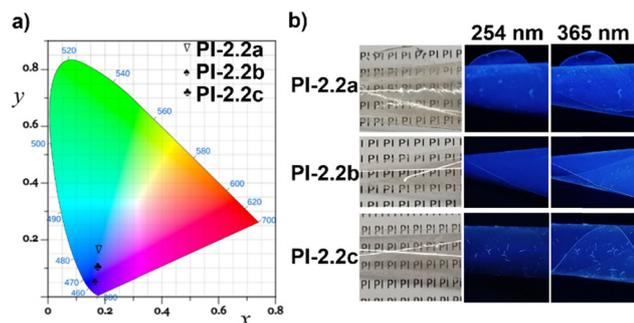
Fig. 7 (a) CIE chromaticity diagram 1931 of emissive PI film series PI-2.2a–c.<sup>46</sup> (b) photographs of PI films under ambient light and a hand-held UV lamp (254 and 365 nm).
