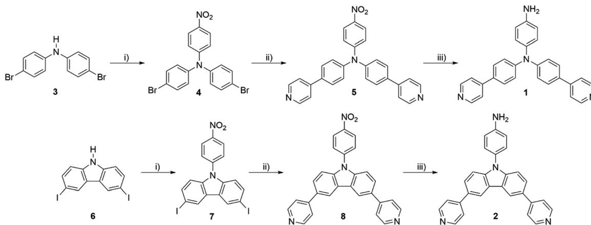
Scheme 1 Synthesis of comonomers **1** and **2**: (i) 1-fluoro-4-nitrobenzene, K<sub>2</sub>CO<sub>3</sub>, DMSO, 145 °C, 12 h; (ii) pyridine-4-ylboronic acid, PdCl<sub>2</sub>(PPh<sub>3</sub>)<sub>2</sub>, Na<sub>2</sub>CO<sub>3</sub>, dioxane/H<sub>2</sub>O (4 : 1), 90 °C, 12 h; (iii) Pd/C, N<sub>2</sub>H<sub>4</sub>·H<sub>2</sub>O, EtOH, 100 °C, 12 h.
