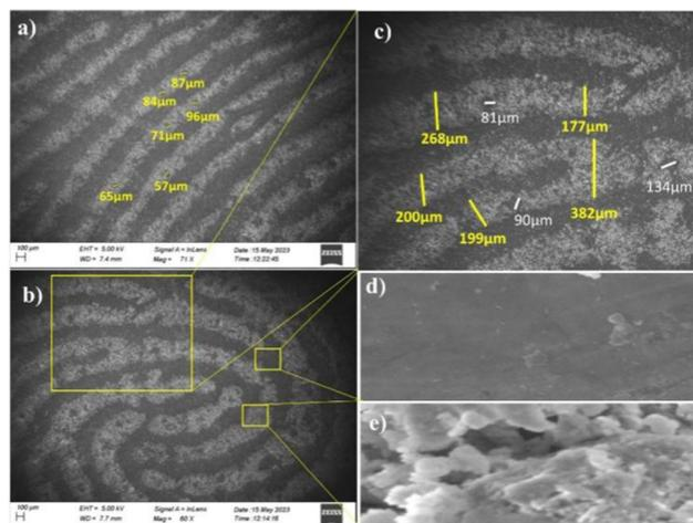
Fig. 7 The micromorphology of LFMs was characterized by FE-SEM; (a) super-resolution of the LFM ridge pattern (insets: yellow-pore size); (b) whorl image; (c) magnified image of a whorl (insets: yellow-ridge width, white lake width); (d) furrow area; (e) ridge area.
