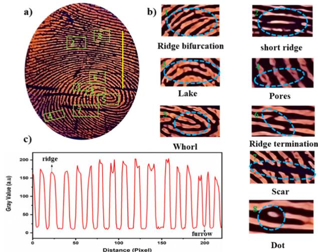
Fig. 5 (a) RGB true colour image of LFM developed by **Py-Pr-OH** on aluminium foil (under 356 nm UV light) using an iPhone13; (b) enlarged image displaying different LFM level (1–3) information such as (1) ridge bifurcation; (2) short ridge; (3) lake; (4) pores; (5) whorl; (6) ridge termination; (7) scar; (8) dot; (c) variation of fluorescence intensity between the fingerprint ridges and furrows across the yellow line (grayscale image).
