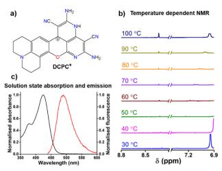
Fig. 4 (a) Chemical structure of DCPC+; (b) temperature-dependent NMR data of DCP\* radical as DCPH in DMSO-d showing generation of new peaks due to conversion to DCPC+ at high temperature; (c) normalized absorbance and emission properties of DCPC\* as DCPC\* in DMSO.
