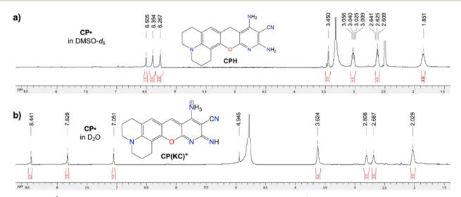
Fig. 5 CP\* radical: <sup>1</sup>H NMR spectra of (a) nonaromatic CPH in DMSO-d<sub>6</sub> and (b) aromatic CP(KC)<sup>+</sup> in D<sub>2</sub>O.
