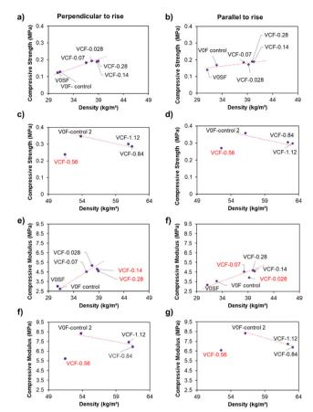
Fig. 5 Specific compressive strength of CNF/RPUF of (a) and (b) low density and (c) and (d) high density and specific compressive modulus of CNF/RPUF of (e) and (f) low density and (f) and (g) high density; both perpendicular and parallel to foam rise (error bars represent standard error and n = 6 samples per direction).
