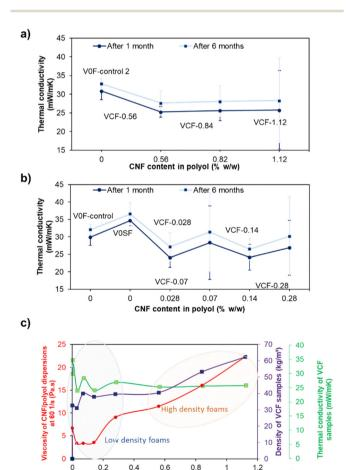
Fig. 6 Initial and aged thermal insulation properties of CNF/RPUF samples (n = 3) at (a) low density and (b) high density (c) correlation of viscosity of polyols and density of RPUF samples with the thermal conductivity of respective RPUF samples.
