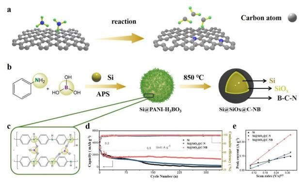
Fig. 9 (a) Schematic diagram of doping manufacturing defects. (b) Synthetic approach of Si@SiO<sub>x</sub>@C-NB, (c) polymer molecular structure, (d) cycling stability for 340 cycles at 0.5 A g<sup>-1</sup> and (e) linear fits for varying sweeping rate CV profiles. 89 Reproduced from ref. 89 with permission from John Wiley and Sons, Copyright 2022.
