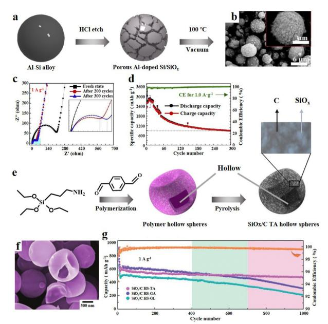
Fig. 3 (a) Schematic diagram of the synthesis of Al-doped porous Si/SiO<sub>x</sub>, (b) SEM images, (c) EIS results and (d) cycling performance at 0.1 A  $q^{-1.51}$ Reproduced from ref. 51 with permission from Elsevier, Copyright 2020. (e) Schematic illustration of the synthetic procedure of SiO<sub>x</sub>/C HS-TA, (f) SEM image and (g) long-term cycling performance at 1.0 A g<sup>-1.54</sup> Reproduced from ref. 54 with permission from John Wiley and Sons, Copyright 2021.
