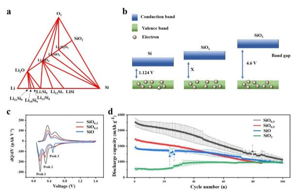
Fig. 4 (a) Ternary phase diagram of Si, O, and Li using density functional theory calculations.<sup>69</sup> Reproduced from ref. 69 with permission from John Wiley and Sons, Copyright 2020. (b) Band gap of Si,  $SiO_x$  and  $SiO_2$ . (c) dQ/dV curves of the 10th cycle data for three  $SiO_x$  films and (d) discharge capacity vs. cycle number of various  $SiO_x$  thin film electrodes over 100 cycles. Reproduced from ref. 70 with permission from American Chemical Society, Copyright 2022.
