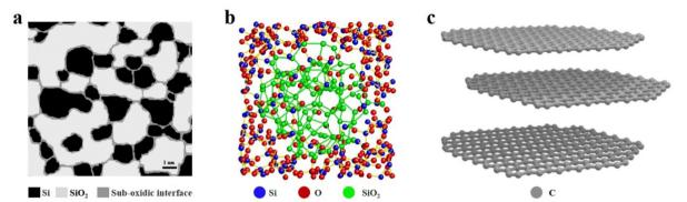
Fig. 2 (a) Schematic illustration of the interface cluster mixture structure of a-SiO. Reproduced with permission.<sup>27</sup> Reproduced from ref. 27 with permission from Elsevier, Copyright 2003. (b) Reconstructed heterostructure model of amorphous SiO.<sup>29</sup> Reproduced from ref. 29 with permission from Springer Nature, Copyright 2016. (c) Crystal structure model of graphite.
