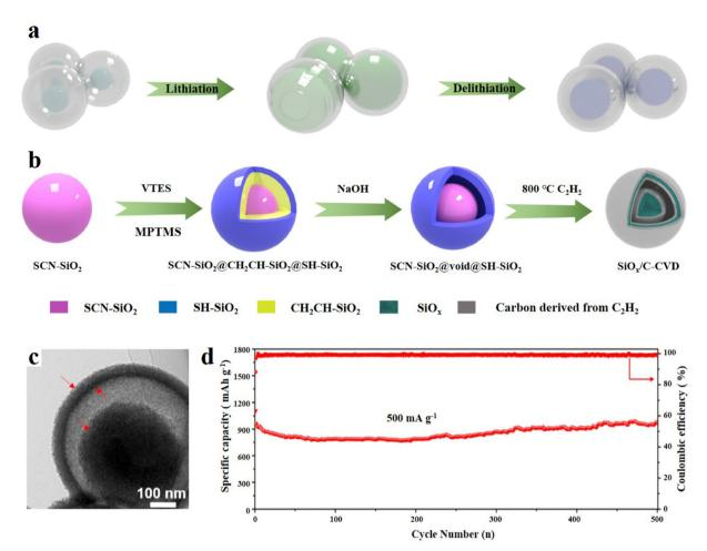
Fig. 6 (a) The evolution of the yolk@shell structure during lithiation/delithiation. (b) Schematic illustration of the preparation of SiO<sub>x</sub>/C-CVD, (c) TEM image and (d) long-term cycling performance at 500 mA g<sup>-1,98</sup> Reproduced from ref. 98 with permission from Elsevier, Copyright 2019
