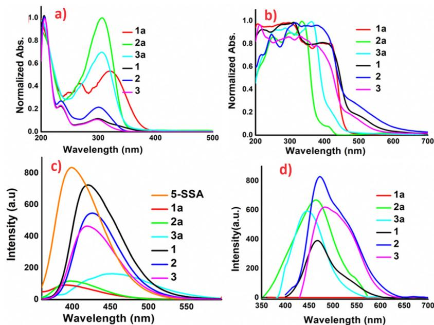
Fig. 3 Photophysical studies: (a) solution phase absorption spectra of  $10^{-3}$  M aqueous solutions, (b) solid phase diffuse-reflectance spectra reported as  $\text{BaSO}_4$  diluted discs, (c) solution phase emission spectra of  $10^{-3}$  M aqueous solutions and (d) solid-state emission spectra reported as  $\text{BaSO}_4$  diluted discs, of **1a–3a** and **1–3**.
