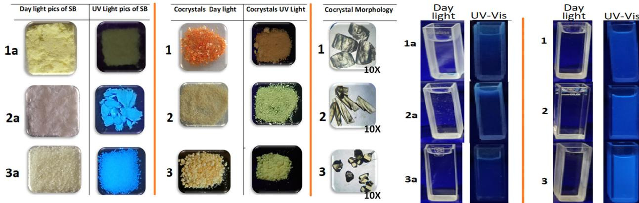
Fig. 2 (Left) Optical images of **1a–3a** and **1–3** recorded under visible and UV exposure and crystal morphologies of **1–3**, at 10× magnification and (Right) optical images of  $10^{-3}$  M aqueous solutions of **1a–3a** and **1–3**, recorded under visible and UV exposure.
