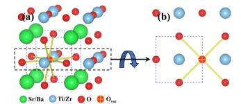
Fig. 2 (a) Possible 8 nearest neighbor jump directions for an oxygen vacancy in either  $TiO_2$  (STO) layer or  $ZrO_2$  (BZO) layer are shown. (b) Normal view for the  $TiO_2$  or  $ZrO_2$  layer depicting the 4 nearest neighbor in-layer jump directions. These 4 directions will be used in the following figures to show the magnitude of activation energy barriers on each side of the heterointerface. The atomic color scheme is given below the figure.
