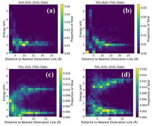
Fig. 7 2D histograms for migration energy barriers at the four interfaces (a)  $SrO-ZrO_2$  (ZrO side), (b)  $TiO_2-BaO$  ( $TiO_2$  side), (c)  $TiO_2-ZrO_2$  ( $TiO_2$  side), and (d) TiO<sub>2</sub>-ZrO<sub>2</sub> (ZrO<sub>2</sub> side). Data are aggregated from all four scenarios performed for each particular interface layer. Distance is calculated using the migration pathway's closest point to the nearest dislocation line.
