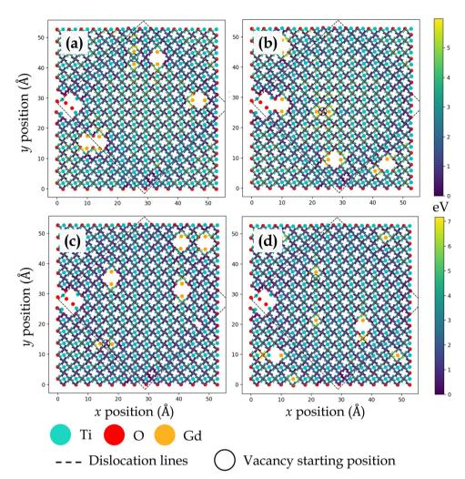
Fig. 6 Activation energy barriers for oxygen vacancy defect migration on the TiO<sub>2</sub> side of the TiO<sub>2</sub>–ZrO<sub>2</sub> interface. In (a)–(c), two Gd<sup>3+</sup> dopants are placed next to the oxygen vacancy in different locations. In (d), each  $Gd^{3+}$  dopant ion is placed isolated, but the total number of dopants and resultant oxygen vacancy concentration is consistent with previous configurations.
