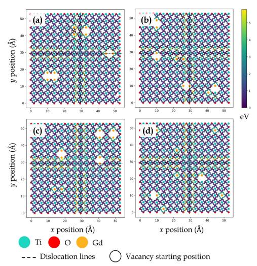
Fig. 4 Activation energy barriers for oxygen vacancy defect migration on the TiO<sub>2</sub> side of the BaO-TiO<sub>2</sub> interface. In (a)-(c), two Gd<sup>3+</sup> dopants are placed next to the oxygen vacancy in different locations. In (d), each Gd<sup>3+</sup> dopant ion is placed isolated, but the total number of dopants and resultant oxygen vacancy concentration is consistent with previous configurations.
