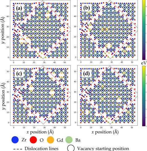
Fig. 5 Activation energy barriers for oxygen vacancy defect migration on the  $ZrO_2$  side of the  $TiO_2-ZrO_2$  interface. In (a)–(c), two  $Gd^{3+}$  dopants are placed next to the oxygen vacancy in different locations. In (d), each  $Gd^{3+}$  dopant ion is placed isolated, but the total number of dopants and resultant oxygen vacancy concentration is consistent with previous configurations.
