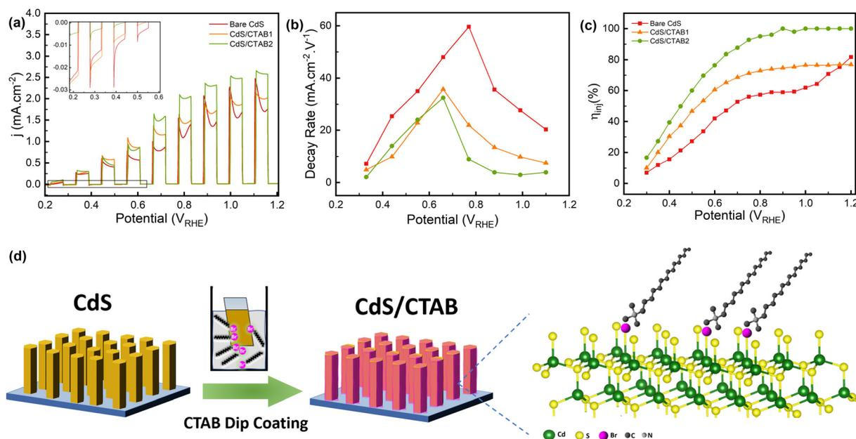
Fig. 2 (a) Chopped illumination LSV, (b) decay rates of the photocurrent after the anodic spike, (c)  $\eta_{\text{inj}}$  of CdS, CdS/CTAB1, and CdS/CTAB2. (d) The schematic representation of the adsorption model of CTAB on CdS after dip coating.
