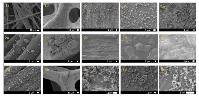
Fig. 4 SEM images for  $Cu_{24}(5-undecoxy-bdc)_{24}$  (#1),  $[Zr_{12}(\mu_3-O)_4(\mu_2-OH)_{12}(Cp)_{12}(m-bdc)_6]Cl_4$  (#2), and UiO-66 (#3) deposited onto carbon paper (a), nickel foam (b), molybdenum foil (c), iron foil (d), or zinc foil (e)
