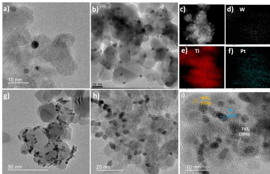
Fig. 2 TEM images of (a)  $\text{TiO}_2/\text{Pt}$  and (b)  $\text{TiO}_2/\text{WO}_3$  materials; (c)  $\text{TiO}_2/\text{WO}_3/\text{Pt}$  (EDX scan image) with its (d) W, (e) Ti and (f) Pt distribution; TEM images of (g)–(i) the  $\text{TiO}_2/\text{WO}_3/\text{Pt}$  heterojunction photocatalyst.
