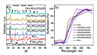
Fig. 1 (a) XRD patterns of  $TiO_2$ ,  $WO_3$  and  $TiO_2/WO_3/Pt$  heterojunction photocatalysts varying their composition and (b) diffuse reflectance spectra of TiO2, WO3 and TiO2/WO3/Pt photocatalysts varying the concentration of WO3.
