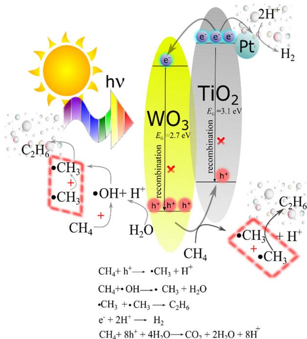
Fig. 7 Energy diagram depicting the charge carrier flux in the  $\text{TiO}_2/\text{WO}_3/\text{Pt}$  ternary photocatalyst under illumination, inhibiting charge carrier recombination towards  $\text{CH}_4$  conversion and  $\text{H}_2$  production.
