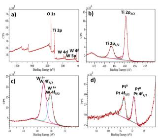
Fig. 3 XPS spectra of the TiO<sub>2</sub>/WO<sub>3</sub>/Pt photocatalyst: (a) typical survey, (b) Ti 2p, (c) W4f and (d) Pt 4f.
