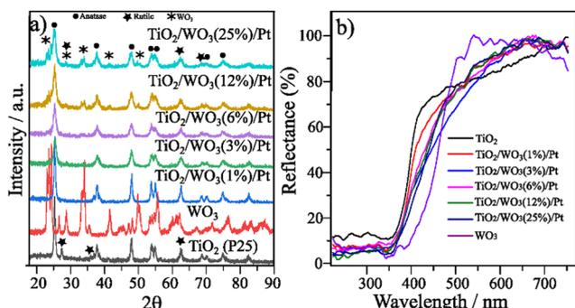
Fig. 1 (a) XRD patterns of TiO<sub>2</sub>, WO<sub>3</sub> and TiO<sub>2</sub>/WO<sub>3</sub>/Pt heterojunction photocatalysts varying their composition and (b) diffuse reflectance spectra of TiO<sub>2</sub>, WO<sub>3</sub> and TiO<sub>2</sub>/WO<sub>3</sub>/Pt photocatalysts varying the concentration of WO<sub>3</sub>.
