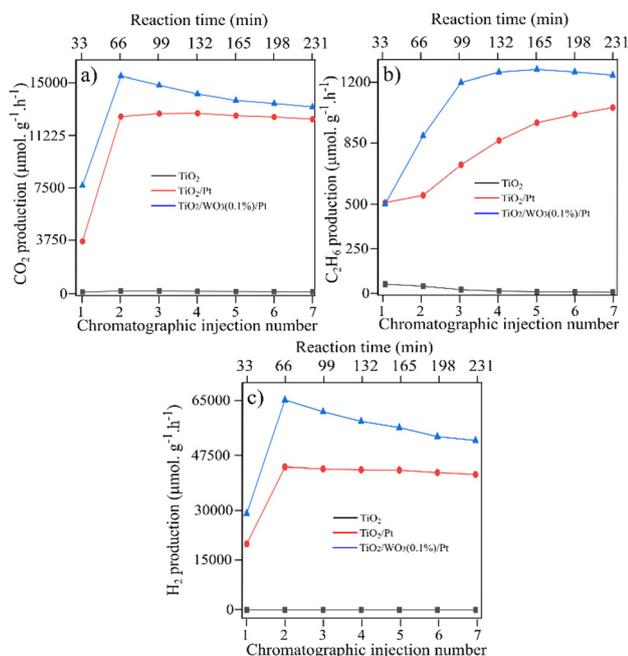
Fig. 5  $\text{CH}_4$  conversion towards the products over  $\text{TiO}_2$ ,  $\text{TiO}_2/\text{WO}_3$  and  $\text{TiO}_2/\text{WO}_3/\text{Pt}$  photocatalysts towards (a)  $\text{C}_2\text{H}_6$ , (b)  $\text{CO}_2$  and (c)  $\text{H}_2$  generation. The  $\text{TiO}_2$  used as support was commercial P25 Degussa.
