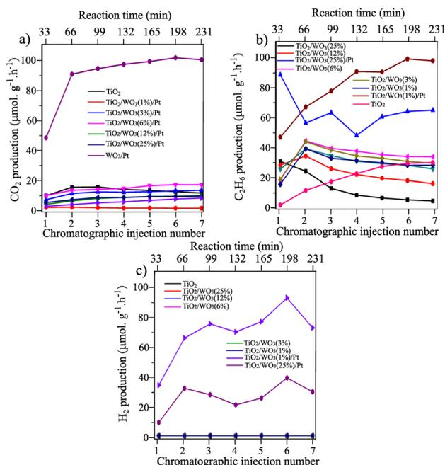
Fig. 4  $\text{CH}_4$  conversion into products over  $\text{TiO}_2$ ,  $\text{TiO}_2/\text{WO}_3$  and  $\text{TiO}_2/\text{WO}_3/\text{Pt}$  photocatalysts towards (a)  $\text{C}_2\text{H}_6$ , (b)  $\text{CO}_2$  and (c)  $\text{H}_2$  generation. The  $\text{TiO}_2$  used as a support was P25 Degussa and the Pt concentration of Pt was set to 0.5%. The time difference between each injection is 33 minutes, corresponding to 4 hours of continuous irradiation.
