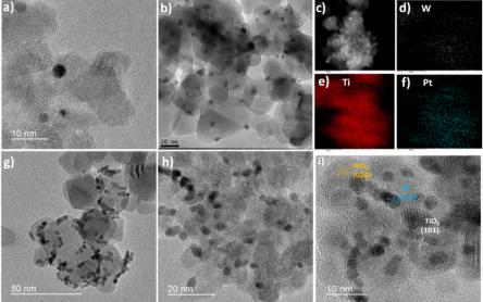
Fig. 2 TEM images of (a) TiO<sub>2</sub>/Pt and (b) TiO<sub>2</sub>/WO<sub>3</sub> materials; (c) TiO<sub>2</sub>/WO<sub>3</sub>/Pt (EDX scan image) with its (d) W, (e) Ti and (f) Pt distribution; TEM images of (g)-(i) the TiO<sub>2</sub>/WO<sub>3</sub>/Pt heterojunction photocatalyst.
