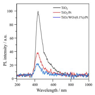
Fig. 6 Room-temperature PL emission spectra of pristine TiO<sub>2</sub> (P25), TiO<sub>2</sub>/Pt and TiO<sub>2</sub>/WO<sub>3</sub>/Pt photocatalysts (excitation wavelength at 265 nm)
