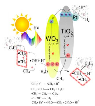
Fig. 7 Energy diagram depicting the charge carrier flux in the TiO<sub>2</sub>/WO<sub>3</sub>/ Pt ternary photocatalyst under illumination, inhibiting charge carrier recombination towards CH<sub>4</sub> conversion and H<sub>2</sub> production
