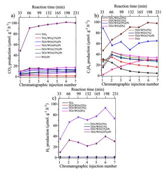
Fig. 4 CH<sub>4</sub> conversion into products over TiO<sub>2</sub>, TiO<sub>2</sub>/WO<sub>3</sub> and TiO<sub>2</sub>/  $WO_3/Pt$  photocatalysts towards (a)  $C_2H_6$ , (b)  $CO_2$  and (c)  $H_2$  generation. The TiO<sub>2</sub> used as a support was P25 Degussa and the Pt concentration of Pt was set to 0.5%. The time difference between each injection is 33 minutes, corresponding to 4 hours of continuous irradiation.
