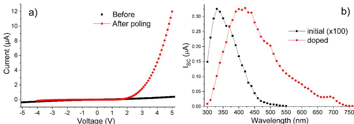
Fig. 7 Optoelectronic properties of **O6** in a  $2 \mu\text{m}$ -thick ITO-ITO cell: (a) dark  $I$ - $V$  curves before and after poling. (b) Spectra of short-circuit photocurrent, measured after poling, for undoped and 10 mol% PCBM doped material.
