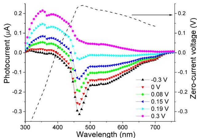
Fig. 9 Photocurrent spectra from PCBM-doped **O6** in a 4  $\mu\text{m}$ -thick cell measured at room temperature and at indicated voltages. The dashed curve shows the value of voltage that results in a zero photocurrent.
