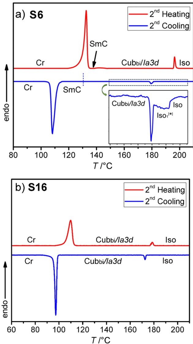
Fig. 3 DSC heating and cooling traces for compounds: (a) **S6** and (b) **S16**. The inset in (a) shows an enlarged view of the Iso-Iso<sub>1</sub><sup>[\*]</sup>-Cub<sub>bi</sub>/Ia<sub>3d</sub> transition on cooling.
