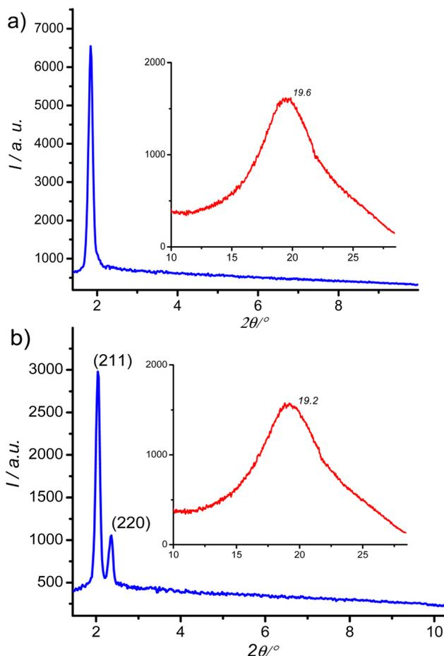
Fig. 5 SAXS patterns of compound **S6** as recorded on cooling: (a) at  $T = 129$  °C in the SmC phase and (b) at  $T = 160$  °C in the  $\text{Cub}_{\text{bi}}/\text{Ia}\bar{3}d$  phase. The insets show the halo peaks detected in the wide-angle region.
