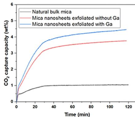
Fig. 8 CO<sub>2</sub> adsorption isotherm at room temperature.
