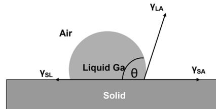
Fig. 3 Sketch of a liquid Ga drop on a solid substrate with the surface free energy and contact angle as described by Young's equation where  $\gamma_{LV}$  = liquid surface free energy,  $\gamma_{SV}$  = solid surface free energy and  $\gamma_{SL}$  = solid/liquid interfacial free energy.
