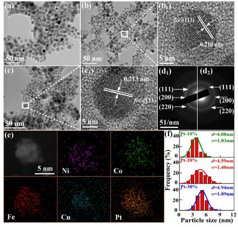
Fig. 5 TEM images of FeCoNiCuPt HEA NPs with Pt contents of (a) 10%, (b) 20%, and (c) 30%. HRTEM images of NPs with Pt contents of (b<sub>1</sub>) 20% and (c<sub>1</sub>) 30%. SAED images of NPs with Pt contents of ( $d_1$ ) 20% and ( $d_2$ ) 30%. (e) Elemental mapping of HEA NPs with Pt contents of 20%. (f) Grain size distributions of HEA NPs.
