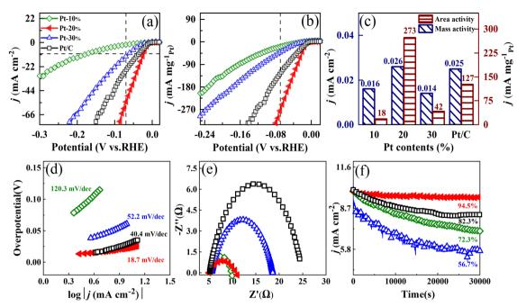
Fig. 7 LSV curves of FeCoNiCuPt HEA NPs with different Pt contents normalized by ECSA (a) and Pt loading (b), (c) Area and mass activity of HEA NPs at -0.07 V. Tafel slopes (d), electrochemical impedance spectroscopy (e), and stability test (f) of HEA NPs. The symbols for different FeCoNiCuPt HEA NPs are consistent, as shown in Fig. 7(a).
