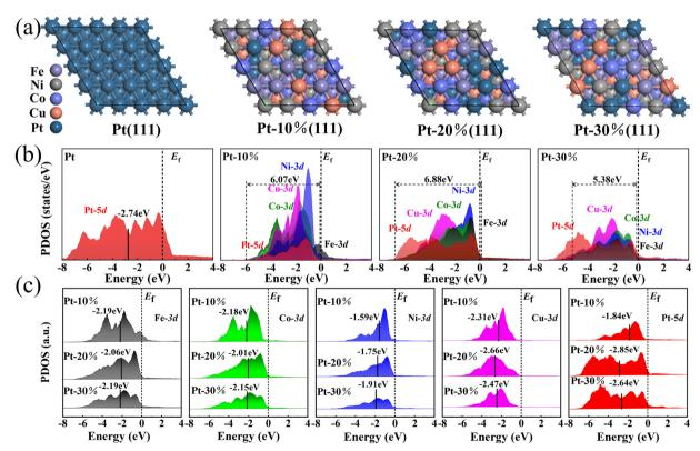
Fig. 9 (a) Top view from the (111) surface of FeCoNiCuPt HEA NPs. (b) PDOS of FeCoNiCuPt HEA NPs with different Pt contents. (c) The Pt contentdependent PDOS and d-band center of Fe, Co, Ni, Cu, and Pt atoms.
