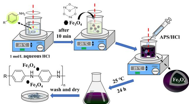
Fig. 1 A diagram of the synthesis of Fe@PANI.
