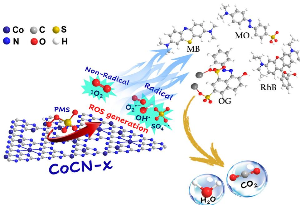
Fig. 11 Possible synergistic degradation mechanism of OG by the CoCN-x/PMS system.
