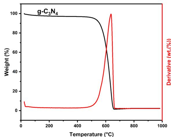
Fig. 1 TGA curve of  $g\text{-C}_3\text{N}_4$ .
