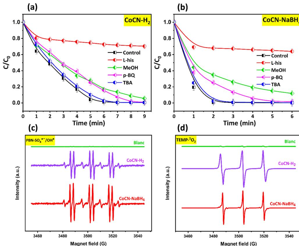
Fig. 10 Scavenger effect experiments on OG removal in (a) the  $\text{CoCN-H}_2/\text{PMS}$  system, and (b)  $\text{CoCN-NaBH}_4/\text{PMS}$  system, and EPR signals of different active free radicals (c)  $\text{PBN-SO}_4^{\bullet-}/\text{OH}^\bullet$  and (d)  $\text{TEMP-O}_2$ .
