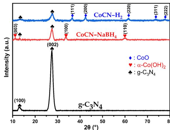
Fig. 3 XRD patterns of CoCN-H<sub>2</sub>, CoCN-NaBH<sub>4</sub>, and g-C<sub>3</sub>N<sub>4</sub>.
