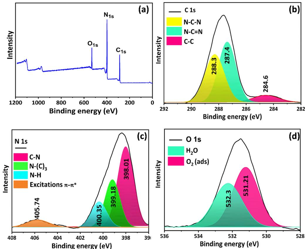
Fig. 2 (a) XPS survey spectrum, and high resolution XPS spectra of (b) C 1s, (c) N 1s, and (d) O 1s of g-C<sub>3</sub>N<sub>4</sub>.
